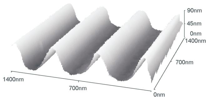
**Fig. 2.** Surface morphology of a periodic structure ablated on a X-cut LiNbO<sub>3</sub> surface with a single pulse at a fluence of 170 mJ/cm<sup>2</sup>, recorded by AFM
