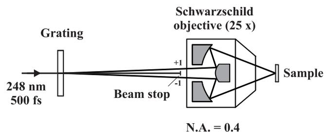
**Fig. 1.** Mask projection set-up with Schwarzschild-type reflective objective
