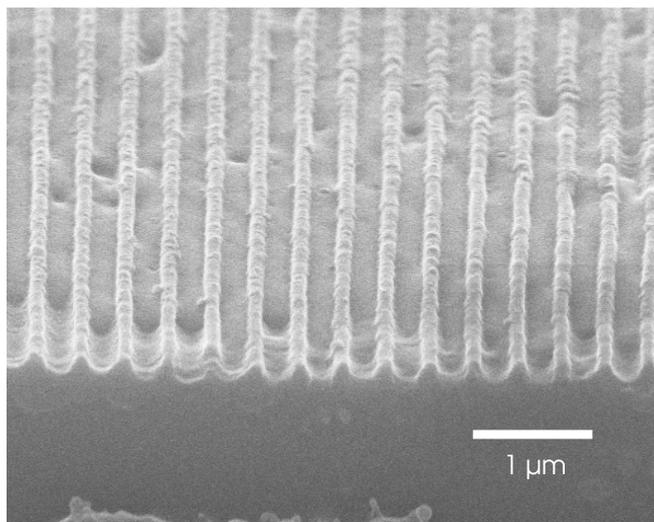
**Fig. 3.** SEM photograph of a grating structure ablated on a X-cut LiNbO<sub>3</sub> surface with 5 pulses at a fluence of 170 mJ/cm<sup>2</sup>
