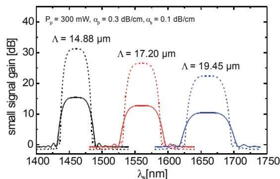
Fig. 2. Calculated small signal gain as function of the wavelength for three different periodicities of the microdomain structure of Ti:PPLN channel guides of 80 mm (solid line) and 160 mm (dashed line) length.
