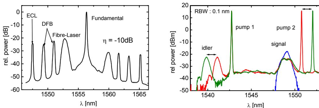
Fig. 1. (left) Output spectrum of a Ti:PPLN wavelength converter for multi-channel operation by cDFG. (right) Output spectra showing all-optical tuning of the idler by the wavelength of pump 2 exploiting cSFG/DFG.
