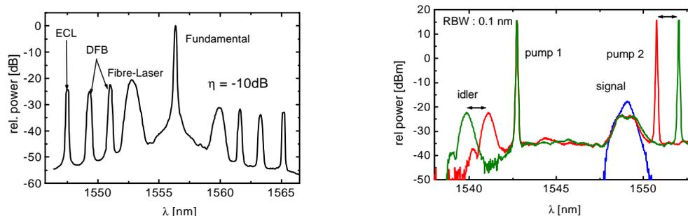
Fig. 1. Left: Output spectrum of a Ti:PPLN wavelength converter for multi-channel operation by cSHG/DFG. Right: Output spectra showing all-optical tuning of the idler by the wavelength of pump 2 exploiting cSFG/DFG.
