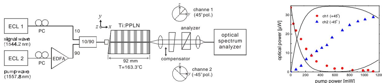
Fig. 2. Left diagram: schematic experimental setup for all-optical polarisation switching. Right diagram: Optical output power in channel 1 and channel 2 versus pump power. Solid lines present the theoretical results.
