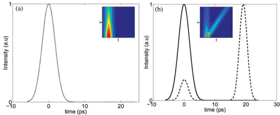
**Figure 5.** Quasi-linear regime. (a) Calculated FF pulse profiles at the input (dotted curve) and output (full curve). (b) Calculated FF (full curve) and SH (broken curve) pulses at output. The temporal slices of the signals are for  $x = 0$ . The insets show the numerical FF (a) and SH (b) temporal evolution in the  $(t, y)$  plane. Here the phase mismatch is  $\Delta kL = 18\pi$  ( $T = 142^\circ\text{C}$ ) and the input intensity is  $I = 1 \text{ MW cm}^{-2}$ .
