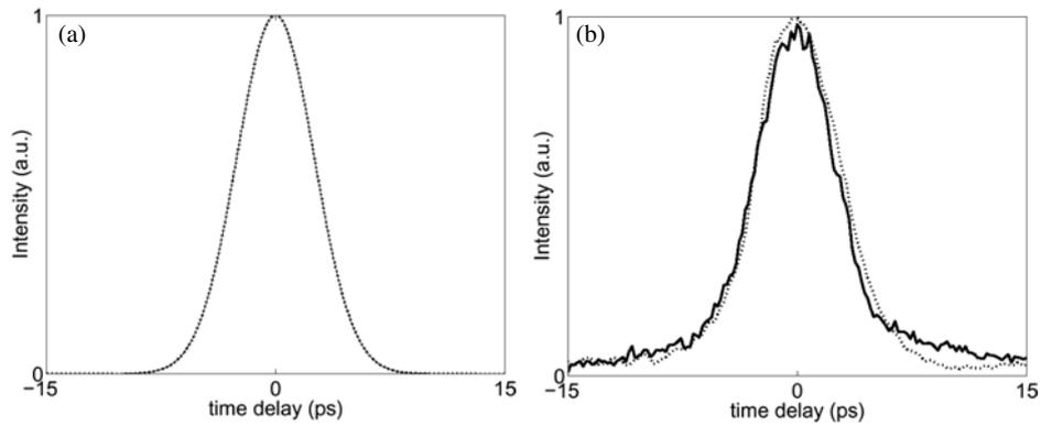
**Figure 7.** Quasi-linear regime. Autocorrelation traces in intensity of the FF at the input (dotted curve) and output (full curve). (a) Numerical simulation, (b) experimental data. Here  $\Delta kL = 18\pi$  ( $T = 142^\circ\text{C}$ ) and the input intensity is  $I = 1 \text{ MW cm}^{-2}$ .
