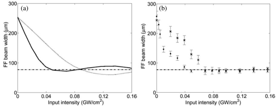
**Figure 3.** FWHM in intensity of the output FF beam versus injected input intensity for different phase-mismatch conditions (or temperatures). (a) Numerical simulations: full curve,  $\Delta kL = 9\pi$ ; dotted curve,  $\Delta kL = 30\pi$ ; chain curve, input width. (b) Experimental data: circles,  $T = 151^\circ\text{C}$  ( $\Delta kL = 9\pi$ ); crosses,  $T = 130^\circ\text{C}$  ( $\Delta kL = 30\pi$ ); chain curve, input width.
