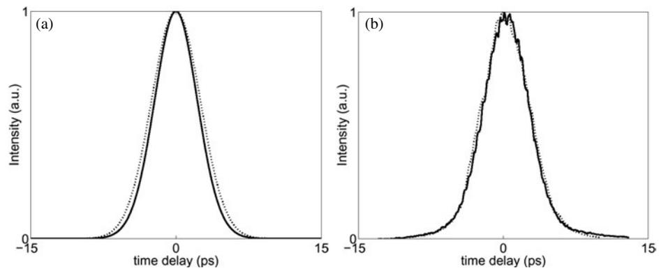
**Figure 10.** Spatial self-trapped regime. Autocorrelation traces in intensity of the FF at the input (dotted curve) and output (full curve) are shown. (a) Numerical simulation, (b) experimental data. Here  $\Delta kL = 18\pi$  ( $T = 142^\circ\text{C}$ ) and the input intensity is  $I = 66 \text{ MW cm}^{-2}$ .
