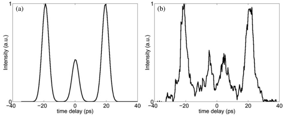
**Figure 6.** Quasi-linear regime. Cross-correlation trace in intensity of the FF and SH signals at output. (a) Numerical simulation, (b) experimental data. Here the phase mismatch is  $\Delta kL = 18\pi$  ( $T = 142^\circ\text{C}$ ) and the input intensity is  $I = 1 \text{ MW cm}^{-2}$ .
