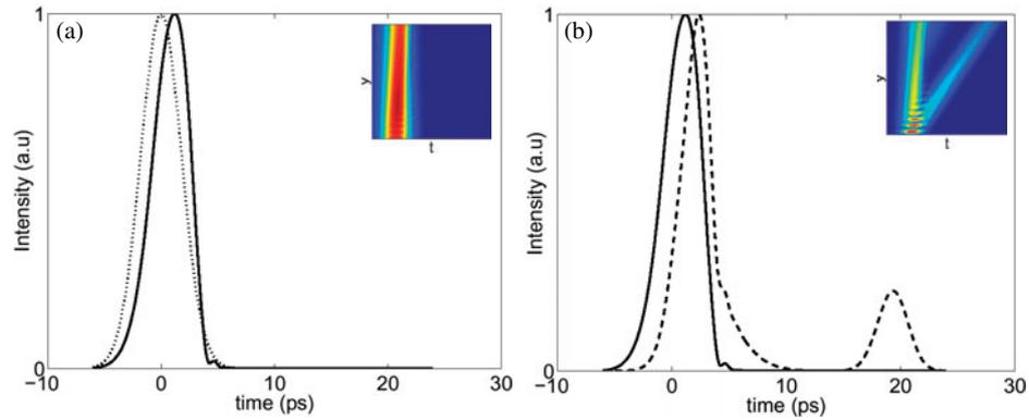
**Figure 8.** Spatial self-trapped regime. (a) Calculated FF pulse profiles at the input (dotted curve) and output (full curve). (b) Calculated FF (full curve) and SH (broken curve) pulses at output. The temporal slices of the signals are achieved for  $x = 0$ . The insets show the numerical FF (a) and SH (b) temporal evolution in the  $(t, y)$  plane. Here the phase mismatch is  $\Delta kL = 18\pi$  ( $T = 142^\circ\text{C}$ ) and the input intensity is  $I = 66 \text{ MW cm}^{-2}$ .
