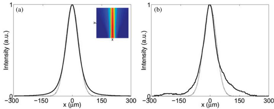
**Figure 2.** Spatial profile of the FF beam, integrated in time, at the input (dotted curve) and output (full curve) in the nonlinear self-trapped regime. (a) Numerical simulations and (b) experimental data. The inset shows the numerical FF beam evolution in the  $(x, y)$  plane. Here the phase mismatch is  $\Delta kL = 18\pi$  ( $T = 142^\circ\text{C}$ ) and the input intensity is  $I = 66 \text{ MW cm}^{-2}$ .
