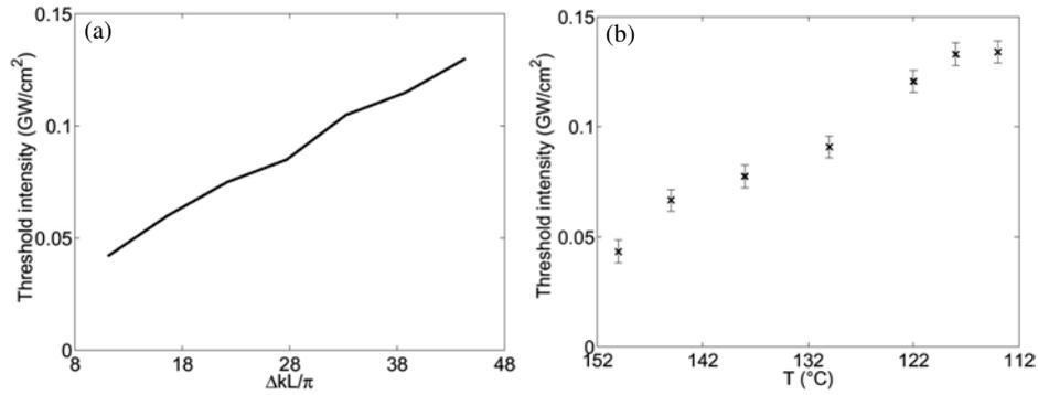
**Figure 4.** Input FF intensity threshold for the generation of self-trapped beams versus phase mismatch (temperature). (a) Numerical simulations, (b) experimental data.
