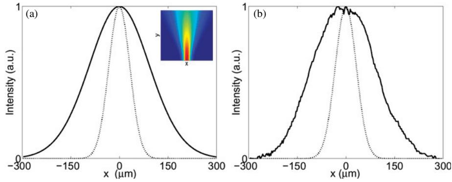
**Figure 1.** Spatial profile of the FF beam, integrated in time, at the input (dotted curve) and output (full curve) in the quasi-linear regime. (a) Numerical simulations and (b) experimental data. The inset shows the numerical FF beam evolution in the  $(x, y)$  plane. Here the phase mismatch is  $\Delta kL = 18\pi$  ( $T = 142^\circ\text{C}$ ) and the input intensity is  $I = 1 \text{ MW cm}^{-2}$ .
