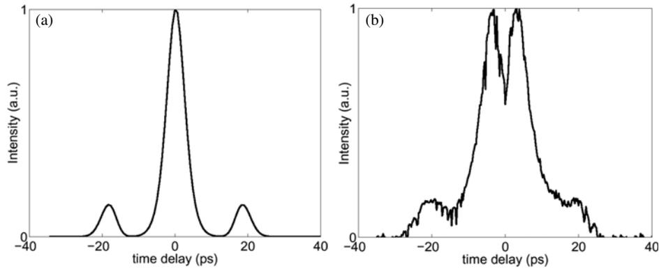
**Figure 9.** Spatial self-trapped regime. The cross-correlation trace in intensity of the FF and SH signals at output is shown. (a) Numerical simulation, (b) experimental data. Here the phase mismatch is  $\Delta kL = 18\pi$  ( $T = 142^\circ\text{C}$ ) and the input intensity is  $I = 66 \text{ MW cm}^{-2}$ .
