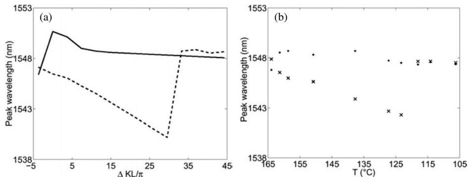
**Figure 14.** Peak wavelength, at the FF and the SH after a two-fold expansion of the SH scale, versus phase mismatch (or temperature) at fixed input intensity. (a) Numerical simulations: full curve, FF signal; broken curve, SH wave. (b) Experimental data: circles, FF signal; crosses, SH wave. Here  $I = 140 \text{ MW cm}^{-2}$ .
