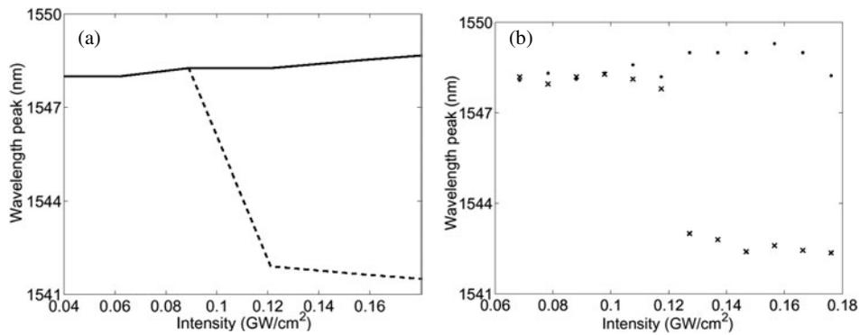
**Figure 13.** Peak wavelength, at the FF and the SH after a two-fold expansion of the SH scale, versus incident intensity at fixed phase mismatch (or temperature). (a) Numerical simulations: full curve, FF signal; broken curve, SH wave. (b) Experimental data: circles, FF signal; crosses, SH wave. Here  $\Delta kL = 18\pi$  ( $T = 142^\circ\text{C}$ ).
