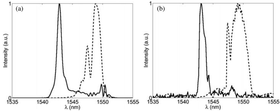
**Figure 12.** Spatial self-trapped regime. Output pulse spectra at the FF (broken curve) and the SH (full curve) after two-fold expansion of the SH scale. Here  $\Delta kL = 18\pi$  ( $T = 142^\circ\text{C}$ ) and the input intensity is  $I = 120 \text{ MW cm}^{-2}$ .
