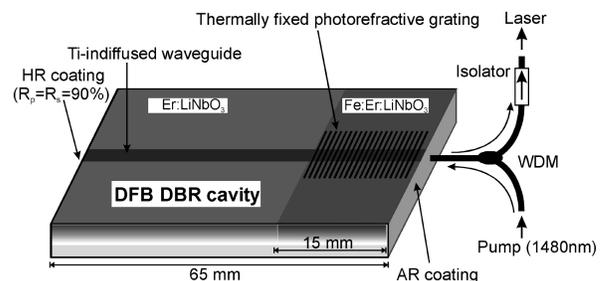
Fig. 1. Schematic structure of DFB–DBR coupled cavity laser in operation: AR, antireflection; WDM, wavelength division demultiplexer.
