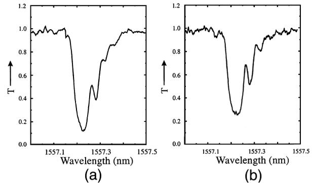
Fig. 2. Normalized transmission characteristics of a fixed ionic grating in TE polarization (a) developed by homogeneous Ar laser illumination ( $250$  mW/cm<sup>2</sup>) and (b) developed by illumination from an array of eight blue LEDs.
