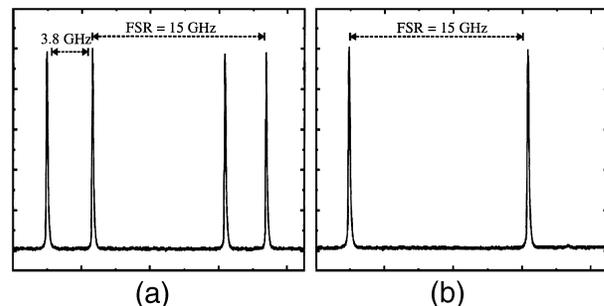
Fig. 4. Measured Fabry–Perot spectra of the laser emission in the DFB–DBR coupled mode of operation at two slightly different temperatures. (a) Simultaneous emission of the two DFB modes with frequencies symmetrical to a pair of DBR cavity modes. (b) Single-frequency emission of one DFB mode in resonance with one DBR cavity mode. FSR, free spectral range of the Fabry–Perot spectrum analyzer.
