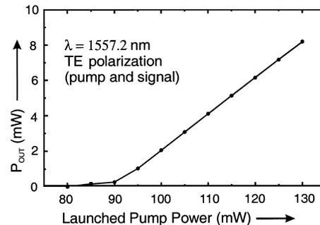
Fig. 3. DFB–DBR coupled cavity laser output power versus launched pump power.
