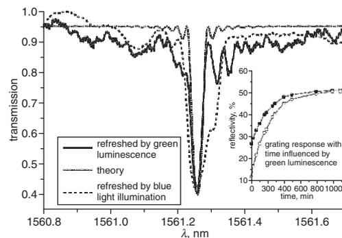
**Fig. 2** Transmission characteristics of 18 mm-long grating in Ti:Fe:Er:LiNbO<sub>3</sub> waveguide for TE-polarised light with 10 pm wavelength resolution
