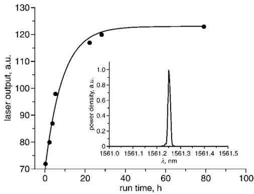
**Fig. 3** DFB-DBR coupled cavity laser stabilisation dynamics with pump laser light ( $\lambda_p = 1480$  nm,  $P = 115$  mW, TE-polarised)
