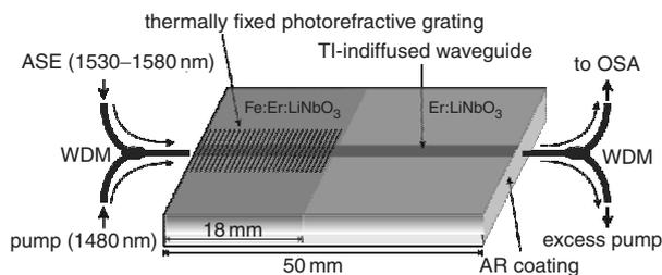
**Fig. 1** Experimental setup for thermally fixed photorefractive grating stabilisation by green luminescence and transmission characteristics measurement
