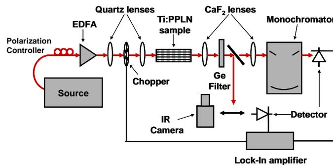
**Fig. 4.:** Schematic experimental setup to investigate integrated OPGs and OPOs.
