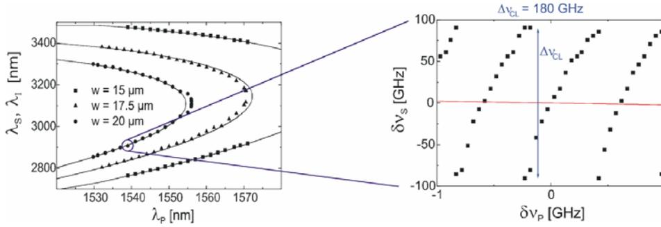
**Fig. 11.** Calculated (solid line) and experimental (dots) tuning characteristics of a doubly resonant OPO with external mirrors as MIR output wavelengths versus the pump wavelength (left) and fine tuning characteristics (right).
