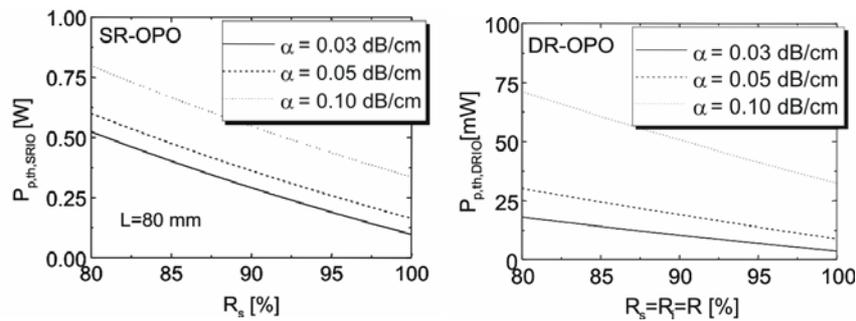
**Fig. 9.** Calculated threshold pump power of a SR-OPO (left) and of a DR-OPO (right) of 80 mm length as function of the reflectivity of the cavity mirrors.
