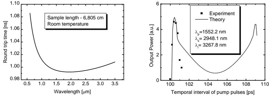
**Fig. 13.** Left: Pulse round trip time versus wavelength in LiNbO<sub>3</sub> waveguides of 6.803 cm length; Right: Calculated (solid line) and experimental (dots) power characteristics of a synchronously pumped DR-OPO with external mirrors as MIR output power versus temporal interval of pump pulses adjusted by the repetition rate of the mode locked pump laser.
