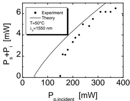
**Fig. 12.** Sum of signal ( $\lambda_s = 2988$  nm) and idler ( $\lambda_i = 3286$  nm) output power of the first IOPO with dielectric mirrors vacuum deposited on the waveguide end faces as function of the incident pump power ( $\lambda_p = 1565$  nm).
