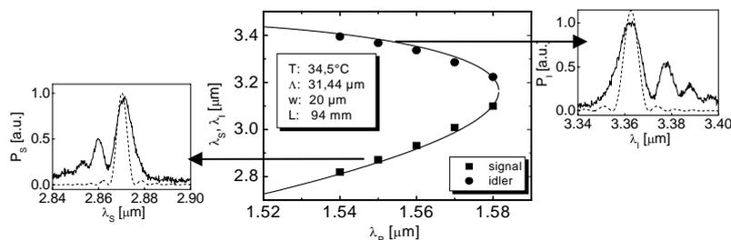
**Fig. 6.** Measured and calculated tuning characteristics of OPF as signal and idler wavelengths versus the pump wavelength in cw-operation (middle diagram) and signal (left graph) and idler (right graph) spectra for the pump wavelength 1548.5 nm as an example.
