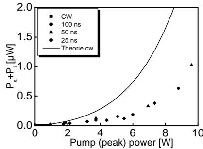
**Fig. 7.** Total OPF output peak power versus coupled pump power (DFB laser,  $\lambda_p=1552$  nm) in a pulsed mode of operation (1 MHz repetition rate) for different pulse width (dots) compared with a theoretical calculation (solid line).
