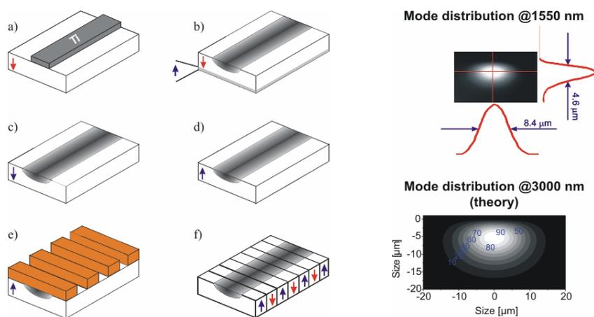
**Fig. 1.** Left: Fabrication of periodically poled  $\text{Ti:LiNbO}_3$  waveguides: a) photolithographic definition of a Ti-stripe and in-diffusion afterwards; b) removal of a domain inverted layer on the +Z face; c) reversal of the spontaneous polarization of the sample as a whole; d) definition of the periodic electrode; e) electric field poling; f) thermal annealing. Right: Measured ( $\lambda=1550$  nm) and calculated ( $\lambda=3000$ nm) mode distributions.
