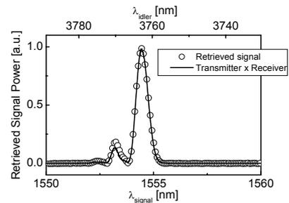
Figure 4: Measured receiver output power versus signal wavelength in the link experiment. For comparison, the product of the measured characteristics of the two modules is shown as well.
