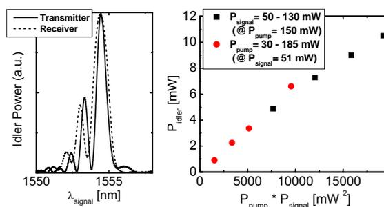
Figure 2: Generated idler power versus signal wavelength (left) and versus the product of signal and pump power (right).
