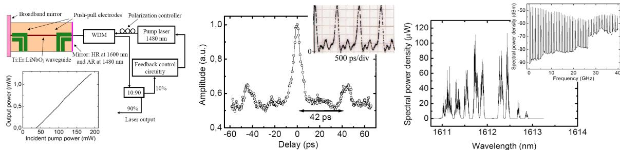
**Fig. 1** Left: Experimental set up with laser power characteristic as inset. Middle: Pulse analysis in the time domain: autocorrelator and sampling scope (inset) results. Right: Pulse analysis in the wavelength domain: optical and radio frequency (inset) spectra of the output.
