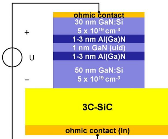
**Figure 1** (online colour at: www.pss-a.com) Schematic drawing of the cubic Al(Ga)N/GaN resonant tunnelling diode structure.
