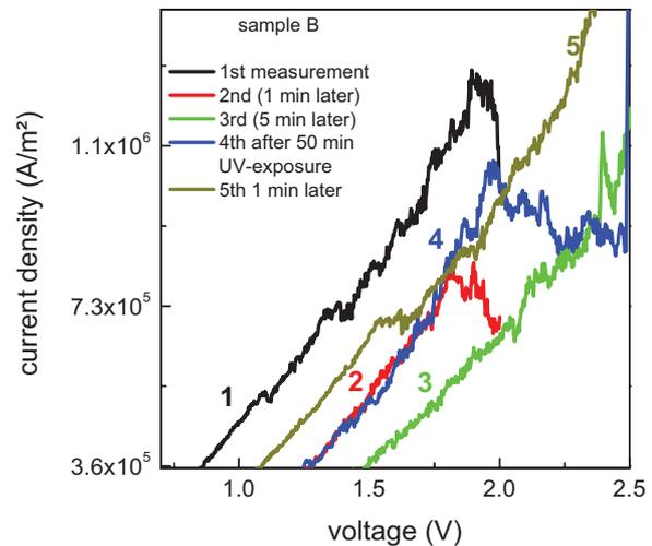
**Figure 5** (online colour at: [www.pss-a.com](http://www.pss-a.com)) Sequenced  $I$ - $V$  characteristics of sample B with vanishing (green and dark yellow curve) and recovering (blue curve) negative differential resistance.
