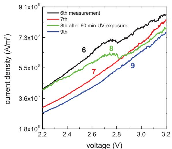
**Figure 6** (online colour at: [www.pss-a.com](http://www.pss-a.com)) Further  $I$ - $V$  characteristics of sample B showing shifted NDR peak and decrease in peak-to-valley ratio.
