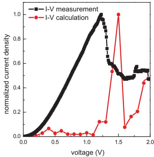
**Figure 3** (online colour at: [www.pss-a.com](http://www.pss-a.com)) Calculated  $I$ - $V$  characteristic of sample A (red dots) in comparison to the measured  $I$ - $V$  curve (black squares).
