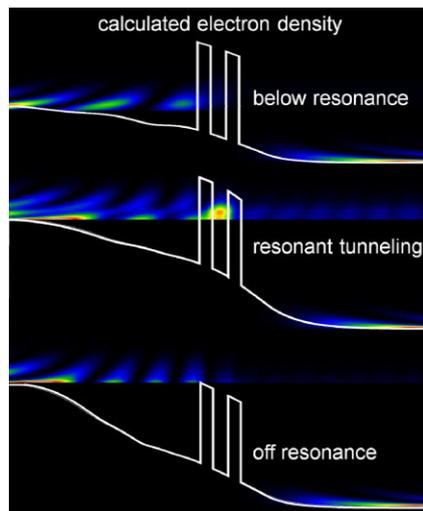
**Figure 4** (online colour at: [www.pss-a.com](http://www.pss-a.com)) Calculated electron density and corresponding band structure for three different bias voltages. Resonant tunnelling occurs for the case of high density inside the QW (middle).
