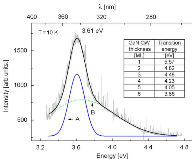
**Fig. 3.** Photoluminescence spectrum of c-GaN droplet QDs. Two overlapping Gaussian shaped emission bands were identified, one at an energy of  $3.61 \pm 0.01 \text{ eV}$ , marked with A, and the other at  $3.64 \pm 0.01 \text{ eV}$ , marked with B. The inset lists the transition energies for various c-GaN quantum wells.
