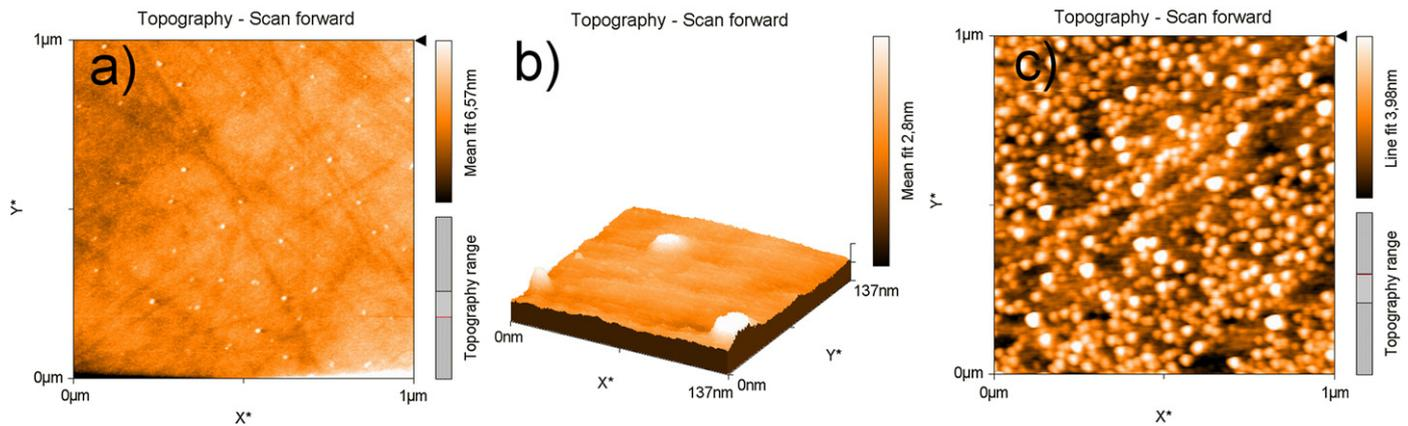
**Fig. 2.** AFM images: (a)  $1 \times 1 \mu\text{m}^2$  GaN QDs grown by method A on c-AlN, the average width of the QDs is 10 nm, the height 2.5 nm and the density  $5 \times 10^9 \text{ cm}^{-2}$ , (b) 3D close-up of GaN QDs in (a), (c)  $1 \times 1 \mu\text{m}^2$  GaN QDs grown by method B on c-AlN, the average width of the QDs is 20 nm, the height 3 nm and the density  $2 \times 10^{11} \text{ cm}^{-2}$ .
