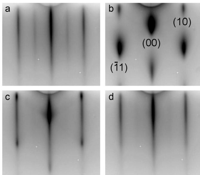
**Fig. 1.** RHEED patterns: (a) reflections of the c-AlN layer, long thin streaks indicate a smooth 2D surface. (b) Reflections of c-GaN droplet QDs, the spotty reflections indicate 3D islands of cubic crystal structure. (c) Reflections of the c-AlN layer after 4 ML QD overgrowth, the smaller FWHM of the spotty reflections indicate partially strained GaN QDs. (d) Reflections of the c-AlN after 30 ML QD overgrowth, long thin streaks indicate a smooth 2D surface.
