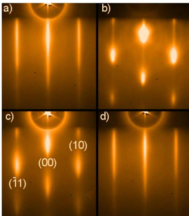
**Figure 1** RHEED patterns: (a) Reflections of the c-AlN layer, long thin streaks indicate a smooth 2D surface. (b) Reflections of c-GaN SK QDs, the spotty reflections indicate 3D islands of cubic crystal structure. (c) Reflections of c-GaN droplet QDs. (d) Reflections of the c-AlN after 30 ML QD overgrowth
