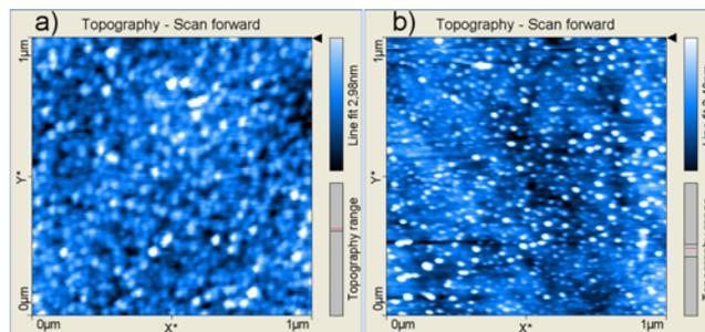
**Figure 2** Atomic force microscopy images: (a)  $1 \times 1 \mu\text{m}^2$  area of the AlN surface covered with SK GaN QDs. The average width of the QDs is 25 nm, the height 3 nm and the density  $1 \times 10^{11} \text{ cm}^{-2}$ , (b)  $1 \times 1 \mu\text{m}^2$  area of the AlN surface covered with DE GaN QDs. The average width of the QDs is 15 nm, the height 2.5 nm and the density  $3 \times 10^{10} \text{ cm}^{-2}$ .
