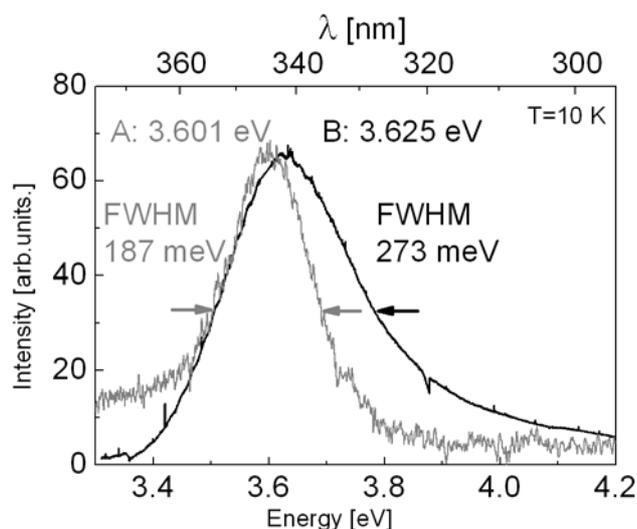
**Figure 3** Photoluminescence spectra: (A) Gaussian shaped emission band of c-GaN SK QDs peaking at an energy of  $3.601 \pm 0.01$  eV. FWHM 187 meV. (B) Gaussian shaped emission band of c-GaN DE QDs peaking at an energy of  $3.625 \pm 0.01$  eV, FWHM 273 meV. A high energy tail indicates a skewed size distribution towards smaller QDs.
