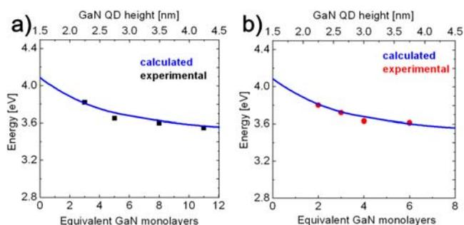
**Figure 4** Correlation between deposited GaN amount, QD height, and QD emission energy. The dots mark the measured QD emission energies of 4 samples. The Graph shows the calculated QD emission energy over QD height relation; (a) shows the relationship for c-GaN SK QDs, (b) shows the relationship for c-GaN DE QDs.
