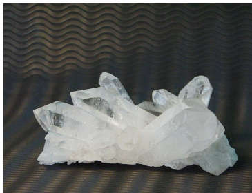
Fig. 1.29 A rock crystals is a well known example for crystal growth. The winning nucleus determines the crystal direction of more than 10^{23} molecules.
