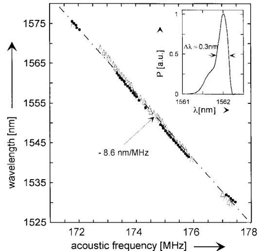
Fig. 6. Emission wavelength of the Ti:Er:LiNbO<sub>3</sub> waveguide laser versus acoustic frequency. Dots: diode-pumped ( $P_p = 110$  mW) laser; triangles: color center laser pumped ( $P_p = 180$  mW) laser. Dash-dotted line: straight line as guide of the eye. Pump polarization: TM. signal output polarization: TE. Inset: emission spectrum of the tunable laser at 1562-nm center wavelength.
