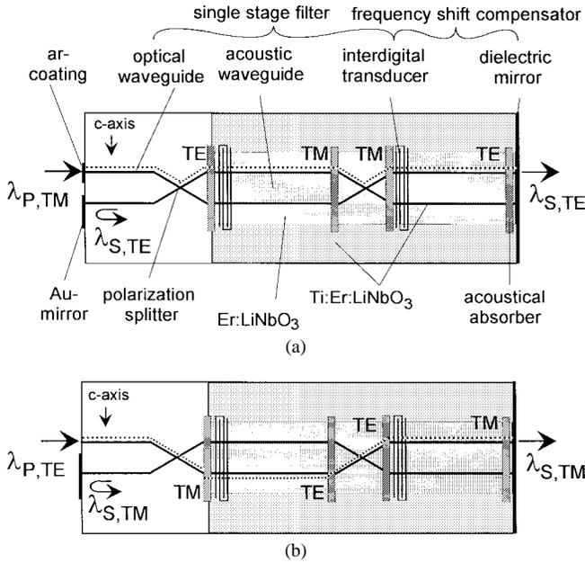
Fig. 1. Schematic diagram of the acoustooptically tunable Ti:Er:LiNbO<sub>3</sub> waveguide laser with a single-stage wavelength filter/frequency-shift compensator combination (a) for TM polarized pump leading to TE-polarized output and (b) for TE-polarized pump leading to TM-polarized output. The path of the pump (P) is given as dotted line. The states of polarization of the circulating resonant signal (S) are indicated by TE and TM within the mode converters.
