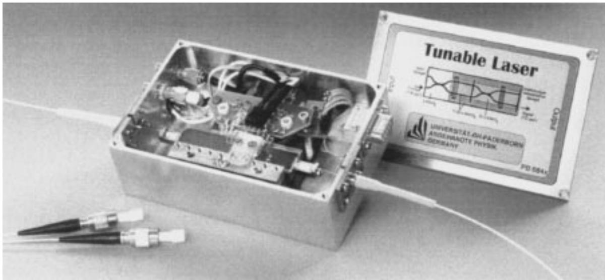
Fig. 4. Photograph of pigtailed and packaged acoustooptically tunable Ti:Er:LiNbO<sub>3</sub> waveguide laser.
