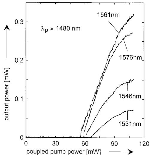
Fig. 5. Output power versus coupled pump power for diode-pumping of the pigtailed and packaged tunable Ti:Er:LiNbO<sub>3</sub> waveguide laser. Pump polarization: TM; signal polarization: TE.
