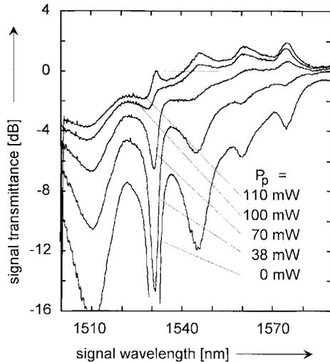
Fig. 2. Signal transmittance through a straight doped waveguide versus wavelength; parameter of the set of graphs is the incident pump power  $P_p$  ( $\lambda_p \approx 1480$  nm). Pump (signal) polarization: TM (TE). The 0-dB line corresponds to the signal transmittance of a straight undoped waveguide.
