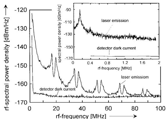
Fig. 7. RF-spectral power density of the detector current versus frequency for laser emission at 1561-nm wavelength. The dc electrical power corresponding to the average optical output power of the tunable laser of 108  $\mu$ W was  $-31.3$  dBm. The spectra have been measured with a resolution bandwidth of 3 kHz at the lower frequencies (inset) and of 500 kHz at the higher frequencies.
