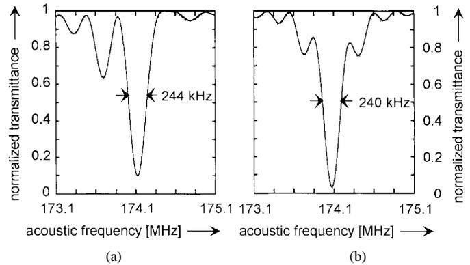
Fig. 3. Normalized transmittance at 1557-nm wavelength versus acoustic frequency for (a) the notch-filter and (b) the frequency shift compensator, measured without pumping of the filter structure. (The notch filter characteristic of the frequency-shift compensator was measured with an external polarizer.)
