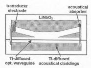
Fig. 1: Integrated acoustooptical polarization converter
