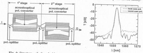
Fig. 4: Structure of the double-stage wavelength filter (left) and measured filter characteristics (right):
