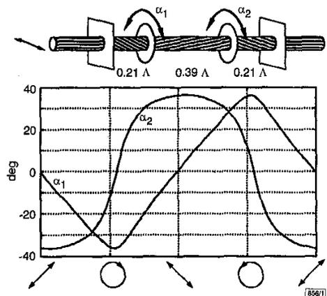
Fig. 1 Twist angle pairs needed for different output polarisations corresponding to half mode conversion of horizontal input polarisation
