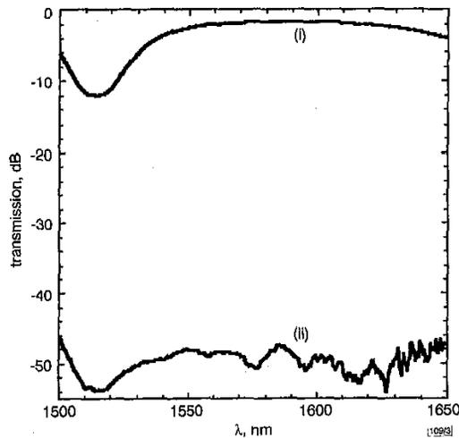
Fig. 3 Fibre-to-fibre transmission spectra of  $1 \times 8$  digital optical switch at 390 mW driving power
