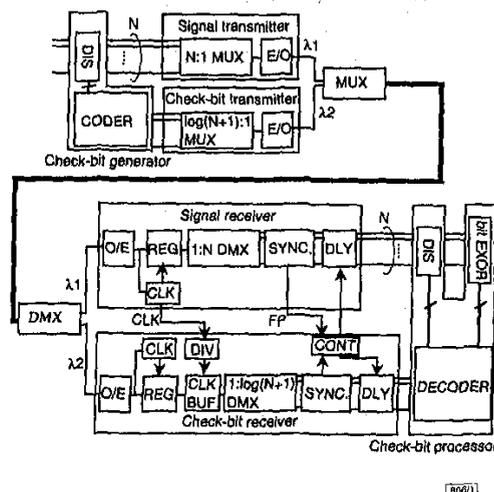
Fig. 1 Proposed system configuration
