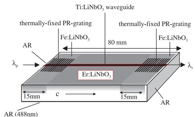
**FIGURE 1** Schematic structure of the Ti:Er:LiNbO<sub>3</sub> waveguide laser with two DBR gratings in Fe-doped sections; AR: antireflection coating
