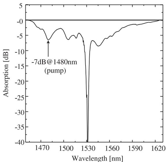
**FIGURE 2** Absorption spectrum of 50-mm-long Ti:Er:LiNbO<sub>3</sub> waveguide section (TE polarisation)
