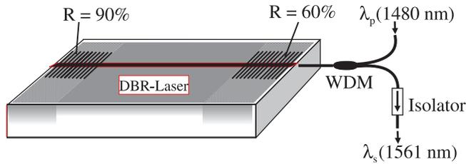
FIGURE 7 Schematic diagram of the DBR laser in operation
