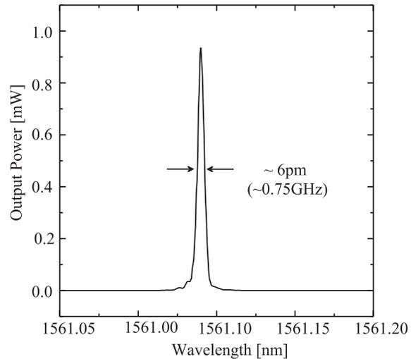
FIGURE 9 Spectral characteristics (TE polarisation) of the DBR laser
