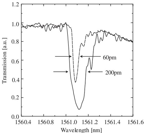
**FIGURE 5** Transmission characteristics (TE mode) of fixed photorefractive gratings of the DBR cavity: *solid line*, high-reflection grating (HR); *dashed line*, output coupler grating
