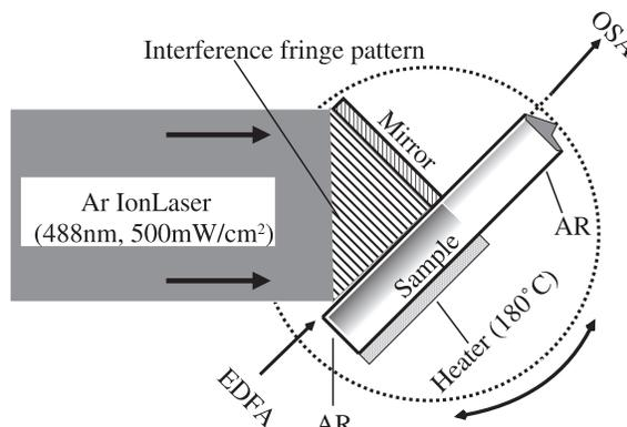
**FIGURE 4** Holographic setup to fabricate fixed photorefractive gratings
