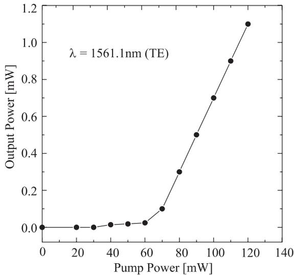
FIGURE 8 Laser output of the DBR laser vs. incident pump power ( $\lambda_p = 1480$  nm; TE polarisation)
