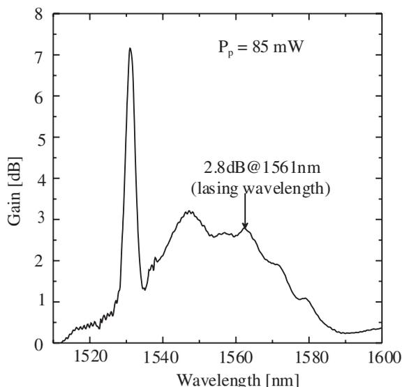
**FIGURE 3** Gain characteristics of 50-mm-long Ti:Er:LiNbO<sub>3</sub> waveguide section; both pump and signal are TE-polarised
