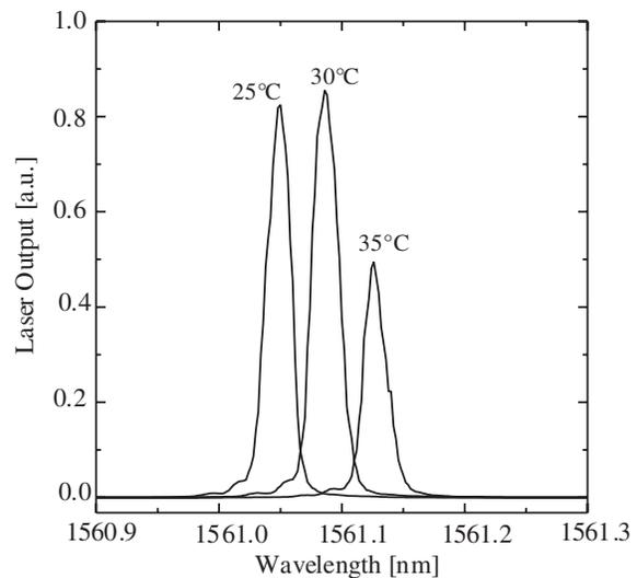
FIGURE 10 Tuning characteristics of the DBR laser; the HR grating is kept at room temperature, while the output coupler grating is temperature-tuned
