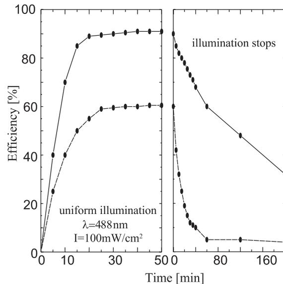
**FIGURE 6** Development and decay characteristics of the gratings: *solid line*, high-reflection grating (HR); *dashed line*, output coupler grating
