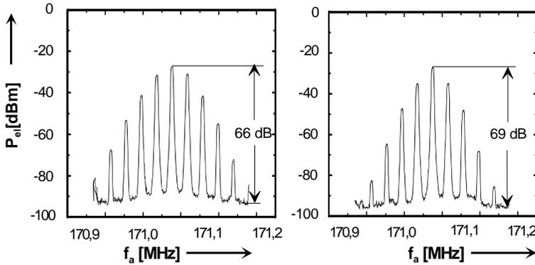
Fig. 4. Measured spectrum (3 kHz resolution) of the heterodyne interferometer signal for operation with a vibrating mirror at 20 kHz with balanced receiver of two detector of type FRM3Z121LT with bandwidth (100 MHz) (*left*) and detector of type FRM3Z621KT with bandwidth (400 MHz) (*right*).
