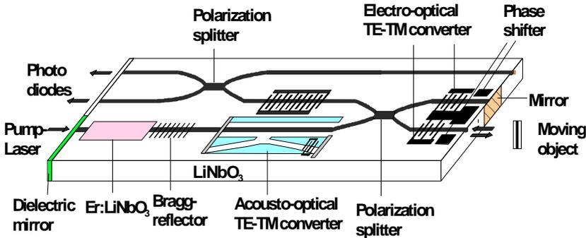
Fig. 5. Monolithic integration of the Ti:Er:LiNb<sub>3</sub> DBR-waveguide laser.
