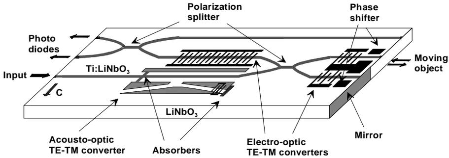
Fig. 1. Scheme of the integrated optical heterodyne interferometer.
