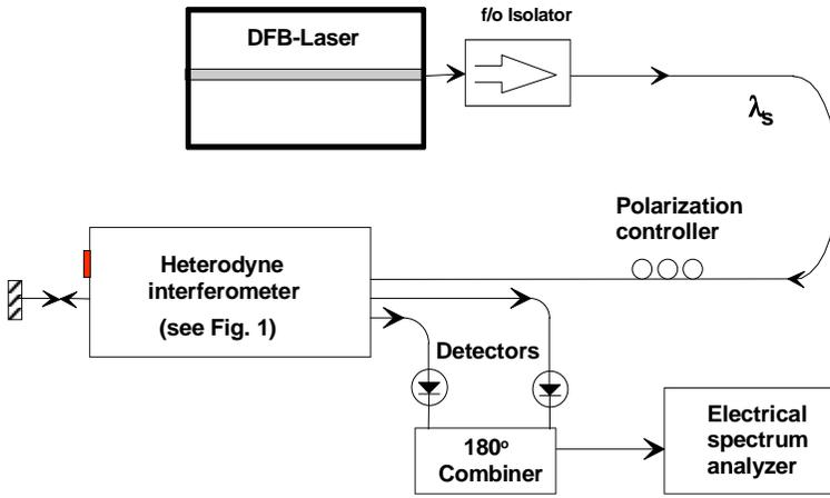
Fig. 2. Set up to characterize the heterodyne interferometer using a DFB Laser diode.
