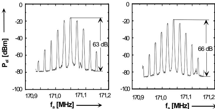
Fig. 3. Measured spectrum (3 kHz resolution) of the heterodyne interferometer signal for operation with a vibrating mirror at 20 kHz with detector of type FRM3Z121LT with bandwidth (100 MHz) (left) and detector of type FRM3Z621KT with bandwidth (400 MHz) (right).
