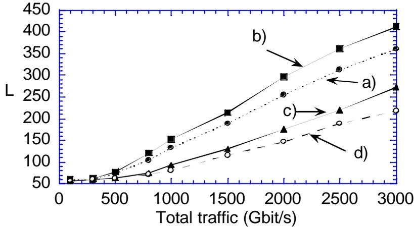
Fig. 8: Number of 40 Gbit/s lightpaths vs distance in links encompassing G.652 fibres, by using: a) transmission with the POC-PRE technique with a  $T_{FWHM}=5$  ps,  $\Delta f=200$  GHz and EDFA, b) POC technique with  $T_{FWHM}=8.5$  ps,  $\Delta f=100$  GHz and EDFA, c) POC technique with  $T_{FWHM}=8.5$  ps,  $\Delta f=100$  GHz and Raman/EDFA, d) ideal propagation.
