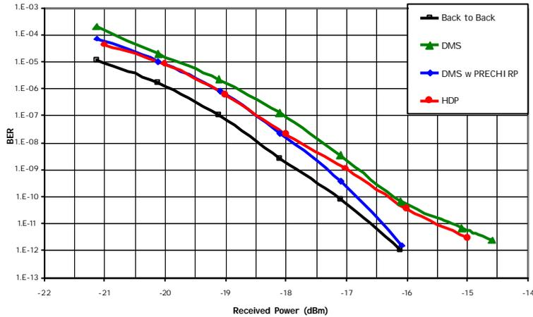
Figure 3: 4 channels 40 Gb/s transmission performance over 5 x 100 km G.652. Channel 2 BER curves with different compensating map: DM and DM with  $-78$  ps/nm pre-chirp (14 dBm/span, 4 dBm/DCU), and HDP (12 dBm/span, 10 dBm/DCU). OSNR is 17 dB for all cases.
