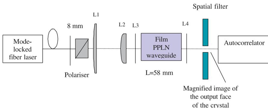
**FIGURE 4** Experimental set-up to investigate spatial self-trapping
