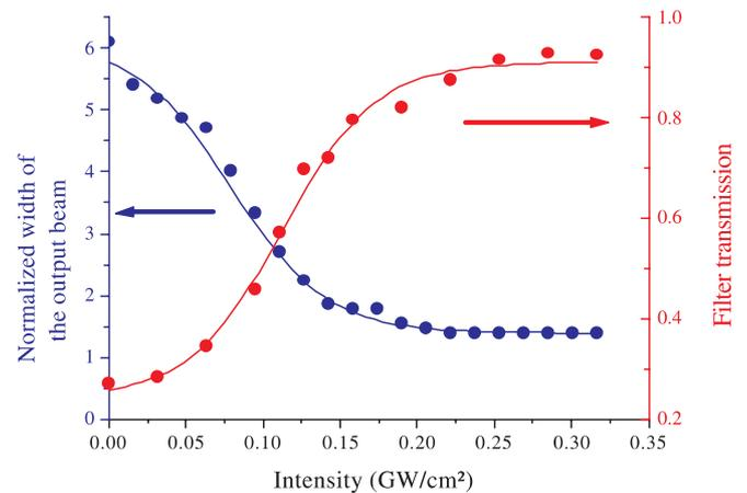
**FIGURE 5** Output beam size and transmittance of the system versus input peak intensity. The temperature was set at 143 °C ( $\Delta kL \sim 15\pi$ ) and the slit width was equal to 0.9 times the input beam width
