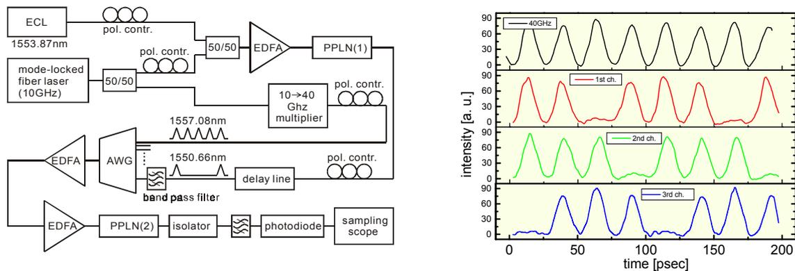
Fig. 2. (left) Experimental setup to demonstrate selective OTDM-channel dropping by SFG. (right) Selective dropping of individual 10 GHz OTDM channels (lower traces) from the 40 GHz OTDM signal (upper trace).
