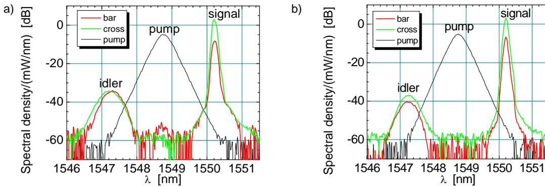
Fig. 2. Measured output spectra from the two coupler arms. a) Pump and signal launched in the bar arm. b) Pump launched in the cross arm. The black line shows the spectrum of the pump versus  $2\lambda_p$ . (pump peak power: 2 W). The low power level of the pulsed signal and idler as compared to the cw peak of the signal is explained by the low repetition rate of the pulsed pump. However, in real applications signal and pump would be generated by two independent synchronized pulsed lasers.
