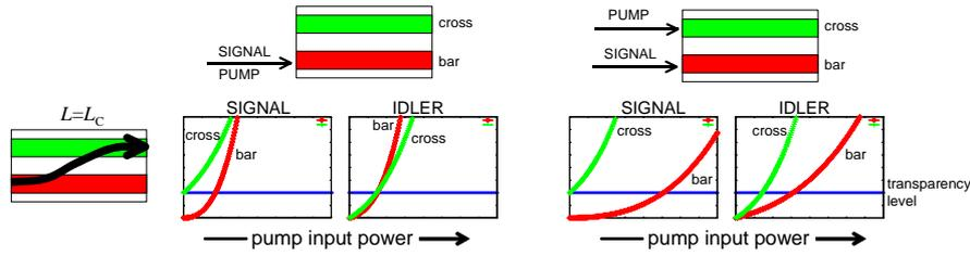
Fig. 1. Parametric interaction in directional couplers. The diagrams show the signal and the idler output for increasing pump input power (arbitrary units) from the two coupler branches. In the left diagrams the pump and the idler are launched in the same coupler arm. The right diagrams show results for pump and signal launched in different waveguides (cw simulations).
