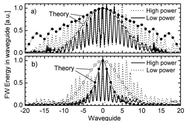
FIG. 4. (a) Nonlinear reinforced beam broadening for in-phase excitation ( $\Delta\beta L = -50\pi$ ,  $L_c = 12.16\text{ mm}$ , FW input peak power of 1.4 kW). (b) Staggered soliton profile ( $\Delta\beta L = -16\pi$ ,  $L_c = 15.7\text{ mm}$ , input peak power of 150 W). Solid and empty circles identify the high- and low-power theoretical data, respectively.
