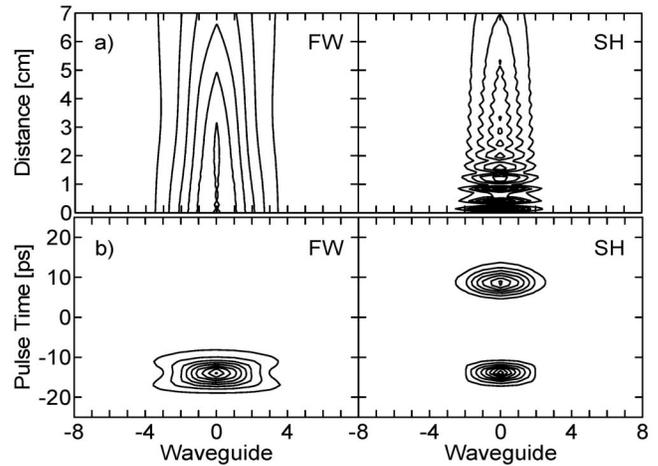
FIG. 3. (a) Simulated evolution of the transverse energy (time integrated) spatial profile of beams excited by a FW input ( $\Delta\beta L = 140\pi$ ,  $L_c = 15.7\text{ mm}$ , FW input peak power of 442 W). (b) Spatiotemporal output distribution of the simulation in (a).
