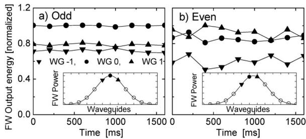
FIG. 5. Time sequence of FW output energies, sampled at intervals of 200 ms, from waveguides in the soliton center ( $L_c = 15.7$  mm,  $\Delta\beta L = 140\pi$ ). (a) Stable output for odd soliton excitation. (b) Unstable output for even excitation.
