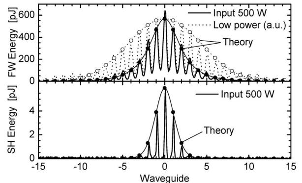
FIG. 1. Spatial pulse energy profile of the two nonlinearly coupled frequency components of an unstaggered odd discrete soliton ( $\Delta\beta L = 140\pi$ ,  $L_c = 15.7$  mm, FW input peak power of 500 W). Dotted lines and open circles show the low-power FW diffracted beam, and solid lines and circles show the soliton. Circles identify theoretical data.
