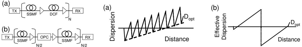
Fig. 1: Experimental setup and effective dispersion map for (a) a conventional DCF aided and (b) an OPC aided transmission system.
