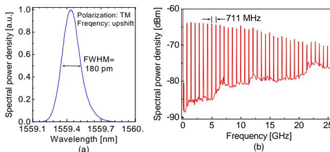
Figure 2: (a) Spectrum of the FSF laser output in TM polarization (frequency upshift); (b) Its RF power spectrum when directly detected by a fast photodiode.
