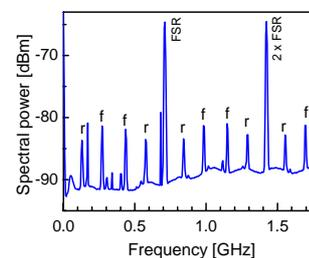
Figure 3: RF-spectrum of the output from a Michelson interferometer with FSF laser as input source.
