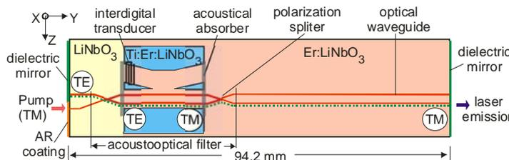
Figure 1: Schematic diagram of the acoustooptically tunable FSF laser in Ti:Er:LiNbO<sub>3</sub> waveguide. X, Y, Z are the crystal axes.
