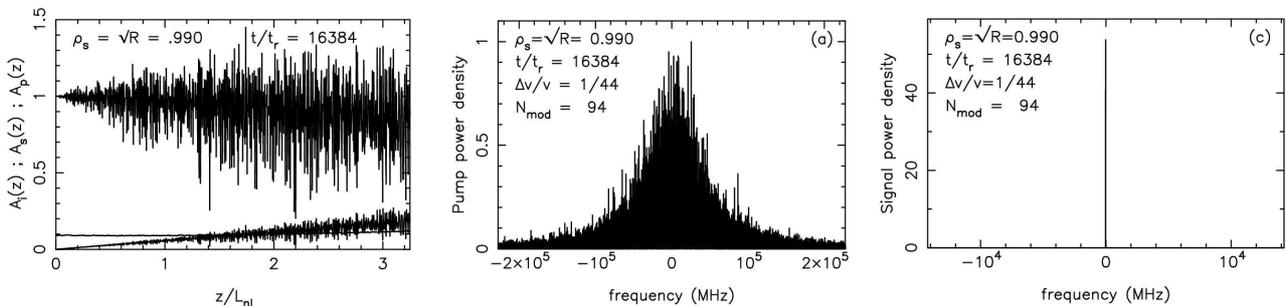
**Fig. 1:** Simulation results for a Ti:LiNbO<sub>3</sub> SR-IOPO ( $\lambda_p = 1.53 \mu\text{m}$ ,  $\lambda_i = 2.51 \mu\text{m}$ ,  $\lambda_s = 3.94 \mu\text{m}$ ): Left: Spatial field amplitude evolution of pump (upper graph), idler and signal waves in the cavity. Middle: Incoherent pump power spectrum ( $\Delta v_p \approx 90 \text{ GHz}$ ). Right: Power spectrum of generated signal ( $\Delta v_s < 2 \text{ MHz}$ ).
