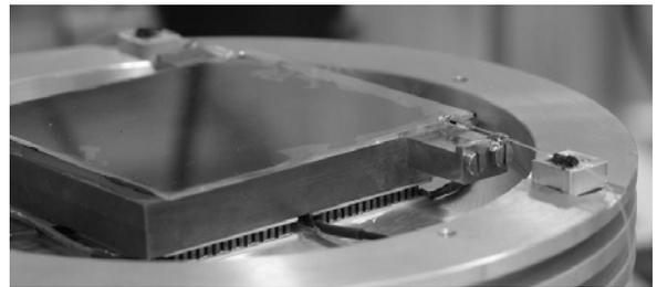
**Fig. 6:** Opened aluminum box with pigtailed ring resonator on a copper base plate, which can be temperature stabilized by a thermoelectric cooler/heater.
