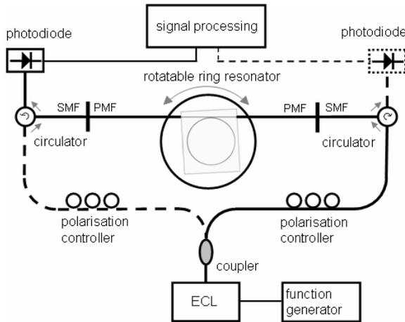
**Fig. 8:** Experimental setup to investigate the ring resonator and to study the Sagnac effect in uni- or bidirectional (dotted) operation. ECL: tunable extended cavity laser. PMF: polarization maintaining fiber. SMF: single-mode fiber
