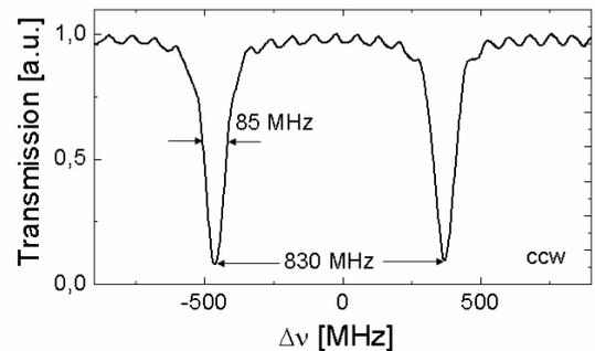
**Fig. 9:** Cw and ccw resonance curves of a ring resonator in bidirectional operation.
