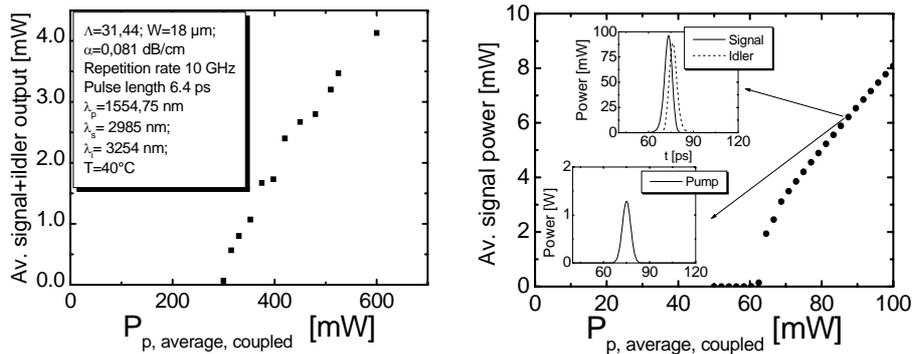
**Fig. 14.** Left: Measured power characteristics of the synchronously pumped OPO as average MIR output power versus the average pump power; Right: Calculated MIR power characteristics versus pump power and output pulses of pump, signal and idler as inset.
