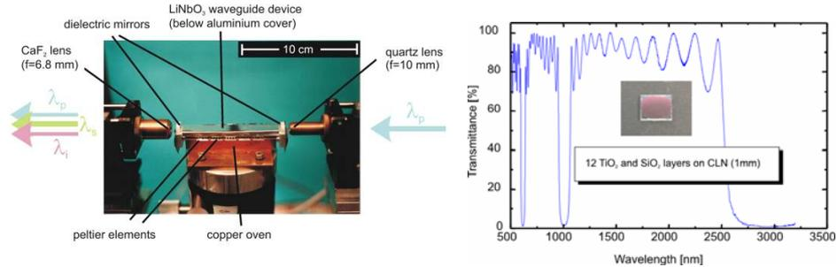
**Fig. 3.:** Left: Ti:PPLN sample in a holder with clamped external mirrors; Right: Transmission of the dielectric cavity mirrors of a doubly resonant MIR-IOPG versus wavelength.
