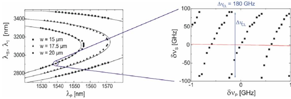
**Fig. 11.** Calculated (solid line) and experimental (dots) tuning characteristics of a doubly resonant OPO with external mirrors as MIR output wavelengths versus the pump wavelength (left) and fine tuning characteristics (right).
