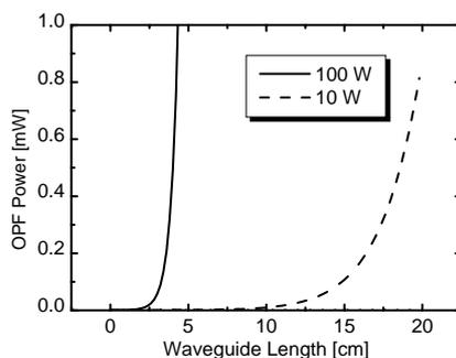
**Fig. 5.** OPF ( $\lambda_s = 2849 \text{ nm}$ ;  $\lambda_i = 3400 \text{ nm}$ ) output power as function of the waveguide length; parameters are the coupled pump power levels ( $\lambda_p = 1550 \text{ nm}$ ).
