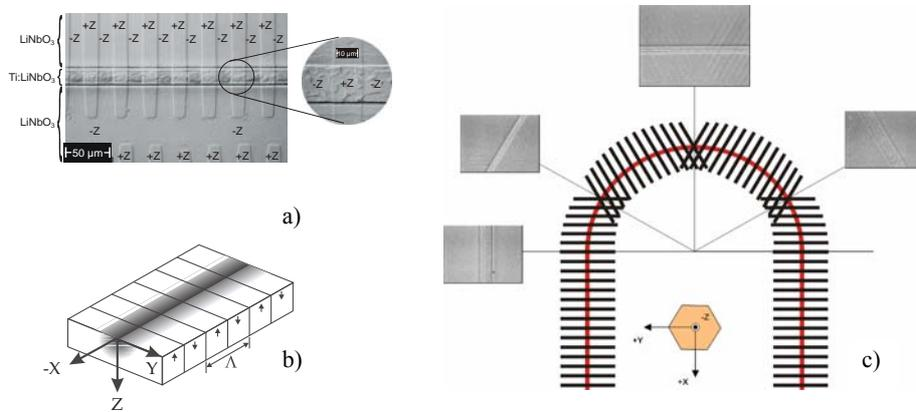
**Fig. 2.** a) Top view of the (selectively etched) ferroelectric domain structure along a straight waveguide; b) Orientation of the optical axes in the sample; c) Top views of parts of the (selectively etched) ferroelectric domain structure oriented parallel to the crystallographic axis.
