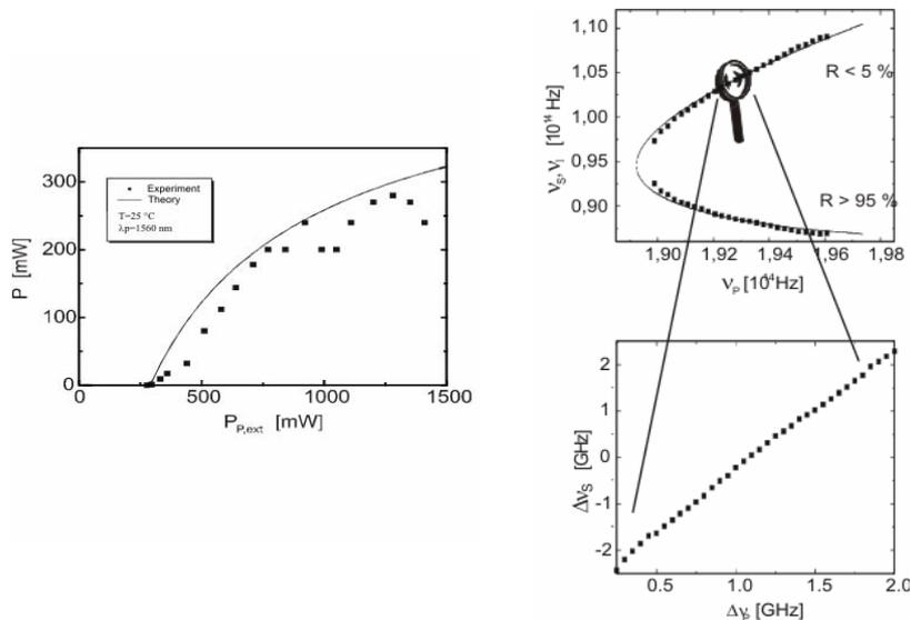
**Fig. 10.** Calculated (solid line) and experimental (dots) power characteristics of a singly resonant OPO with external mirrors as an average MIR output power versus the average pump power (left) and coarse and fine tuning characteristics (right).
