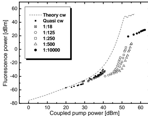
**Fig. 8.** Total OPF output (peak) power versus coupled pump (peak) power in a pulsed mode of operation (6.4 ps pulses of different duty cycle as given in the inset) compared with results of a theoretical analysis (dotted line).
