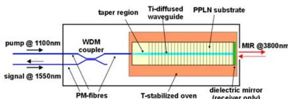
Figure 1: Schematic drawing of the transmitter / receiver modules. Only the receiver module has a dichroic mirror (AR for the MIR, but HR for the pump) to enable signal regeneration by backwards co-directional propagation of both pump and idler waves.
