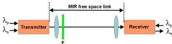
Figure 3: Scheme of the all-optical link from the C-band to the MIR and back to the C-band again.  $F$ : filter to suppress pump and signal radiation of the transmitter.
