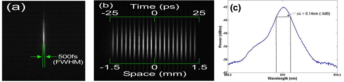
Fig. 2: (a) T-S converted signal pulse image with 500fs FWHM, (b) 20 spatial pulse images distributed throughout the T-S processor time window (composite image) and (c) SFG narrowband spectrum centered at 810nm with a  $-3$  dB bandwidth of 0.14 nm (= 64 GHz).
