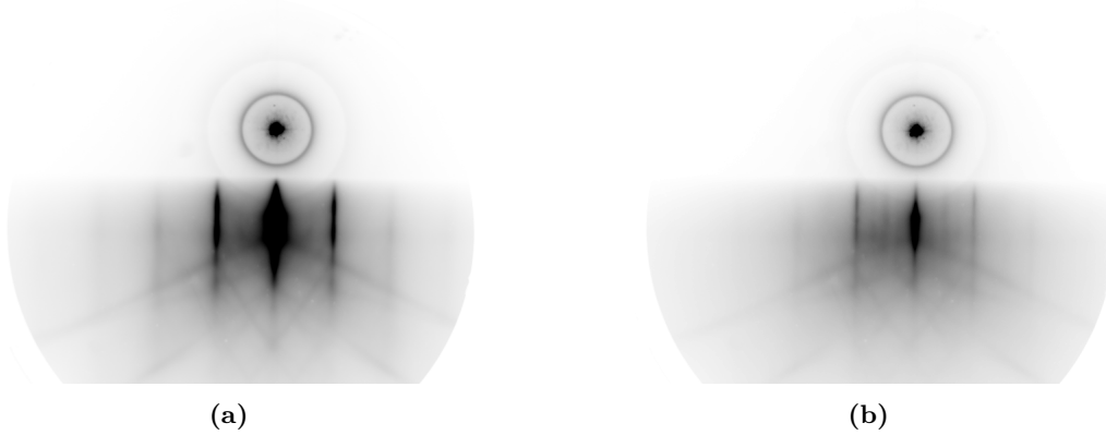
Figure 3.2: RHEED diffraction pattern of a 3C-SiC substrate surface (a) before and (b) after the Al deoxidation procedure at 890 °C.
