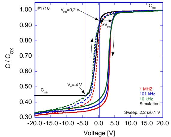
**Figure 1** Hysteresis C-V curves of a cubic GaN MOS structure measured at frequencies of 1 MHz, 100 kHz and 10 kHz. The full black curve shows a simulation of the ideal structure.
