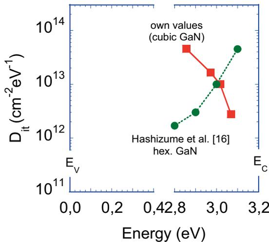
**Figure 3** Interface density  $D_{it}$  vs. energy within the band gap of a cubic  $\text{SiO}_2/\text{GaN}$  MOS structure. (red squares own data, green full circles data from Ref. [16]).
