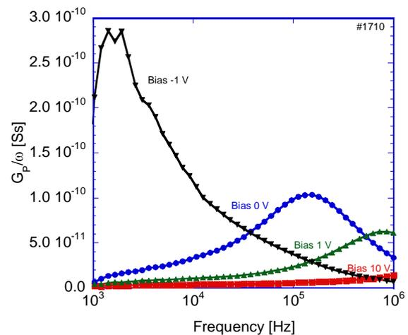
**Figure 2** Conductance  $G_p/\omega$  versus frequency curves of a cubic GaN MOS structure at several biases.
