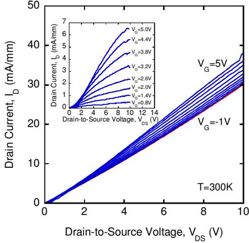
**Figure 1.** Drain current  $I_{DS}$  vs. drain source voltage  $V_{DS}$  of HFET A. The inset shows the same measurement curves corrected for the drain current at  $V_{GS} = -1$  V.
