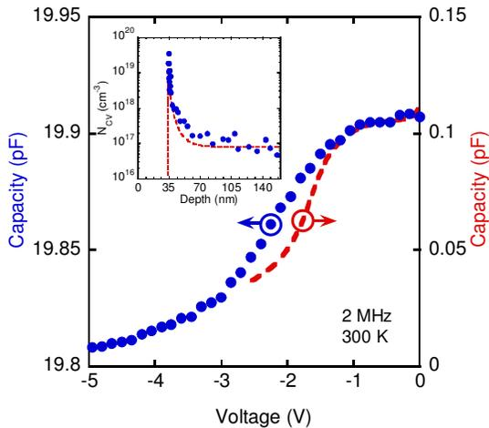
**Figure 3.** CV characteristics of HFET B measured on the gate contact at 2 MHz confirming the presence of an electron channel at the AlGaIn/GaN interface. The inset shows a carrier density profile  $N_{CV}$ . The red dashed lines are CV curves calculated using a Poisson-Schrödinger model.
