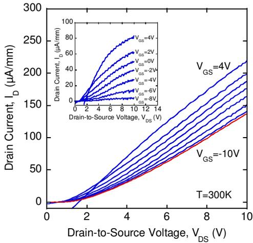
**Figure 2.** Static output characteristics of the HFET B. The inset shows the same measurement curves corrected for the drain current at  $V_{GS} = -10$  V.
