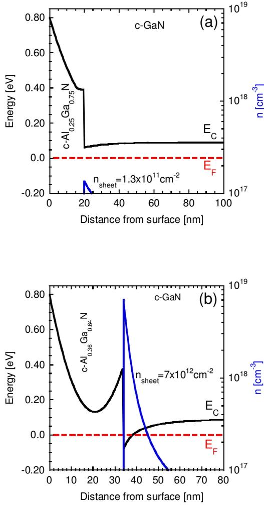
**Figure 4.** Calculated conduction band edge and the electron concentration versus distance from surface at  $V_{GS}=0V$  for (a) Sample A and (b) Sample B.
