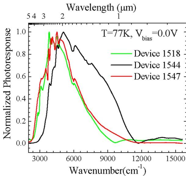
FIG. 1. (Color online) The photoresponse spectra measured for four different devices at 77 K and under zero bias voltage.
