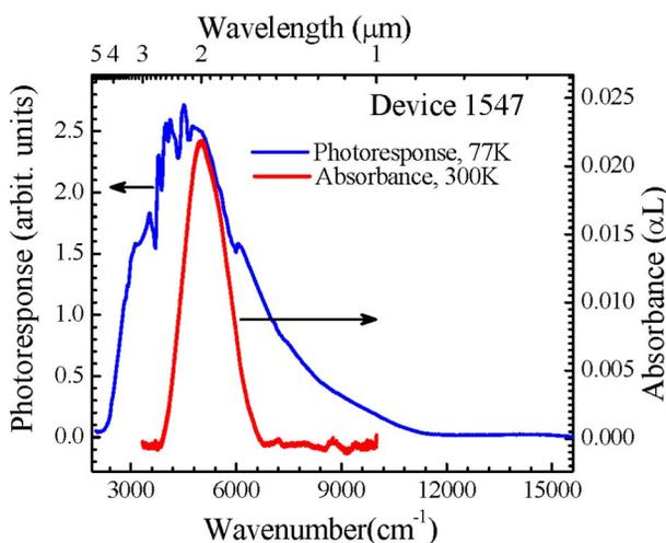
FIG. 2. (Color online) The photoresponse and optical absorbance spectra of device 1547 measured at 77 and 300 K, respectively.
