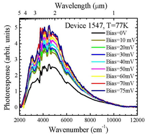
FIG. 3. (Color online) The photoresponse spectra of device 1547 measured at 77 K under different bias voltages.
