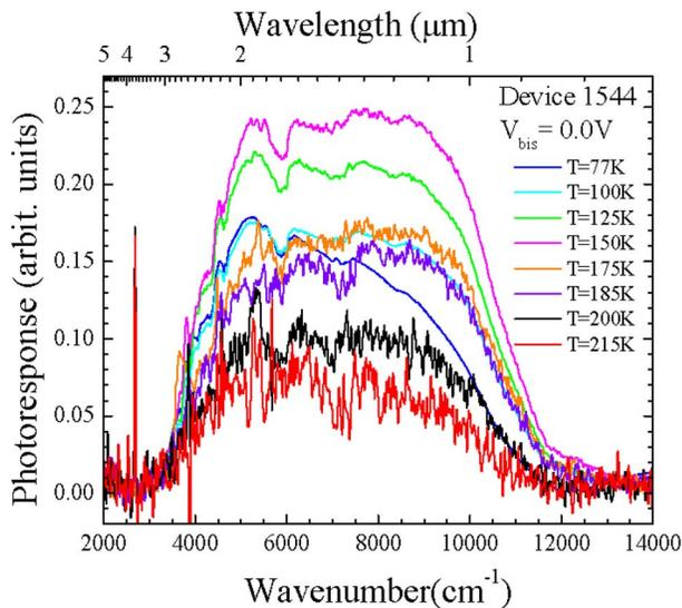
FIG. 4. (Color online) The photoresponse spectra of device 1544 measured at different temperatures under zero bias voltage.
