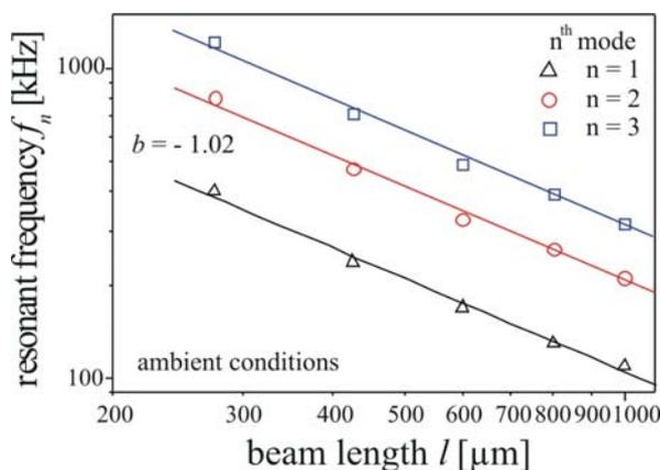
**Figure 4** Resonant frequency  $f_n$  of the  $n^{\text{th}}$  flexural mode versus beam length on double-logarithmic scales. Measurements were carried out for 5  $\mu\text{m}$  wide single layer beams under ambient conditions.
