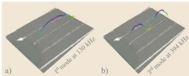
**Figure 3** Exemplary mode shapes of a) the first and b) the third out-of-plane flexural resonance of a 800  $\mu\text{m}$  long and 5  $\mu\text{m}$  wide GaN-resonator under electrostatic actuation monitored by a laser-Doppler vibrometer.
