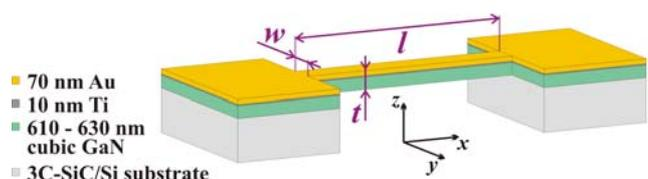
**Figure 1** Schematic drawing of the basic resonator geometry.
