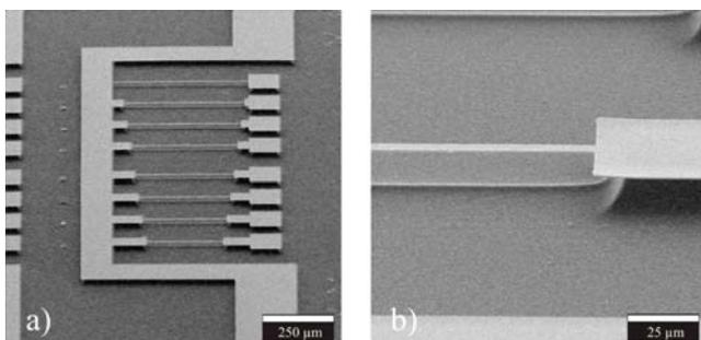
**Figure 2** a) Bird's eye view of a processed GaN resonator array for electrostatic actuation and b) close up view of a GaN beam for magnetomotive actuation.
