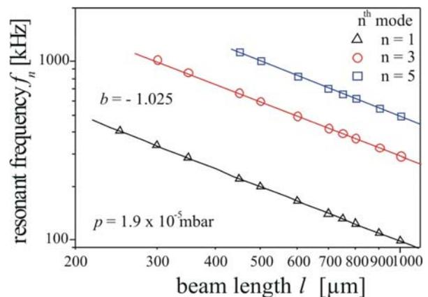
**Figure 5** Resonant frequency  $f_n$  of the  $n^{\text{th}}$  flexural mode versus beam length on double-logarithmic scales. Measurements were carried out for 5  $\mu\text{m}$  wide multi layer beams under vacuum conditions.
