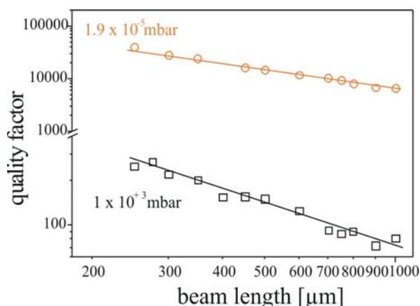
**Figure 6** Quality factor  $Q$  at different levels of ambient pressure and resonant frequency  $f_n$  at a pressure of 0.01 mbar versus beam length. Measurements were carried out for 5  $\mu\text{m}$  wide multi layer beams.
