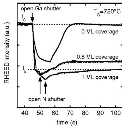
FIG. 3. RHEED intensity transient measured during the growth of *c*-GaN, which started after opening the *N* source. The RHEED intensity measured during growth yields the amount of excess Ga (indicated in the figure) on the *c*-GaN surface. The Ga fluxes are  $4.4 \times 10^{14}$ ,  $3.2 \times 10^{14}$ , and  $1.2 \times 10^{14} \text{ cm}^{-2}$  for the coverages of 1, 0.8, and 0 ML, respectively.
