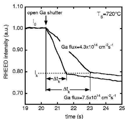
FIG. 2. RHEED intensity transients for two different Ga fluxes as indicated in the figure. After a transition time  $\Delta t_k$  a kink in the transients is observed. Calculating the amount of Ga absorbed (flux times  $\Delta t_k$ ) we find that the kink indicates the adsorption of 1 ML Ga on the *c*-GaN surface.
