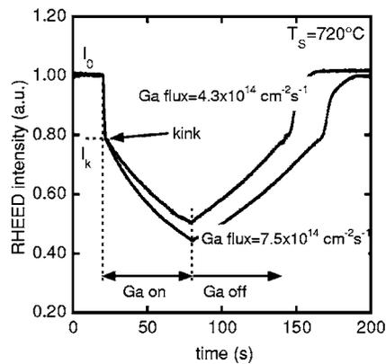
FIG. 1. Intensity of a reflected high energy electron beam (RHEED intensity) vs time measured during the evaporation of Ga onto *c*-GaN at a substrate temperature of 720 °C. The Ga fluxes are indicated.
