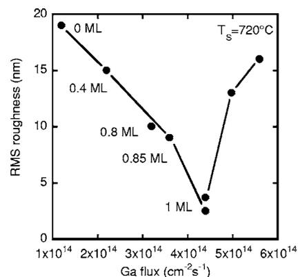
FIG. 4. rms roughness of *c*-GaN layers measured by  $5 \times 5 \mu\text{m}^2$  AFM scans vs Ga flux during growth. The corresponding values of the Ga coverage during growth are also included. Minimum roughness is obtained with an excess coverage of 1 ML. The line is a guide for the eyes.
