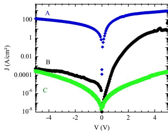
**Figure 5** Current density of the fabricated samples plotted versus the applied voltage. Sample A is the reference sample (blue diamonds), sample B is the sample with UID asymmetric MQW structures (black circles) and sample C contains carbon doped asymmetric MQW structures (green squares).
