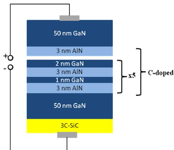
**Figure 1** Schematic drawing of the IV-measurement arrangement. Samples B (undoped) and C (carbon doped) consist of a 50 nm c-GaN buffer followed by 5 asymmetric (1 nm/2 nm) c-GaN quantum wells with (3 nm) c-AlN barriers.
