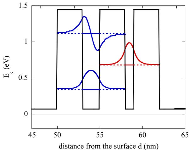
**Figure 3** Conduction band edge and quantized electron states for the first pair of a 2 nm c-GaN QW and 1 nm c-GaN embedded between 3 nm thick c-AlN barriers. The electron wave functions are also plotted. The solid line at 0 eV marks the Fermi level.
