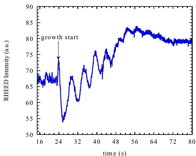
**Figure 2** RHEED intensity transient during the initial growth of c-AlN:C. The oscillations indicate a two-dimensional atomically smooth growth. The growth rate of 0.2 ML/s was obtained from the oscillation period.
