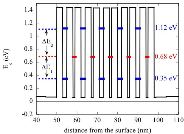
**Figure 4** Conduction band edge as a function of the distance from the surface. The quantized electron states within the QW structure are also shown (blue for 2 nm QWs, red for 1 nm QWs).
