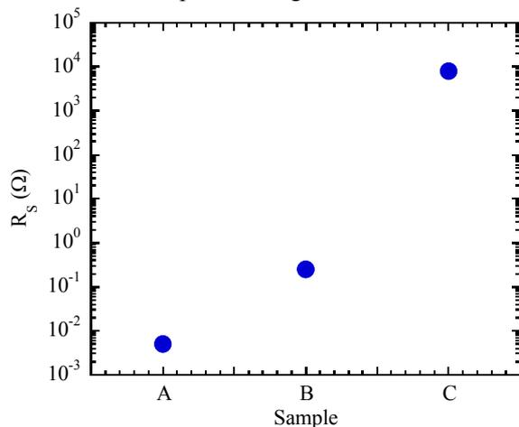
**Figure 6** Serial resistivity  $R_s$  of the fabricated samples A, B and C. The values were obtained from the linear increase of the current vs. voltage characteristics in forward direction.
