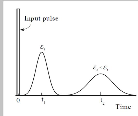
FIGURE 5.18 Carrier diffusion in the Haynes-Shockley experiment in which the input signal is a rectangular narrow pulse applied at point A in Fig. 5.17. The minority carrier pulse is received at point B in Fig. 5.17 at two different electric field values.
