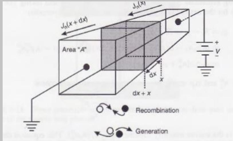
**FIGURE 5.15** A sketch of a sample used to illustrate the derivation of the continuity equation. The four processes that occurred in the segment with thickness  $dx$  are recombination, generation, flow-in current density  $J_n(x)$ , and flow-out current density  $J_n(x + dx)$ .
