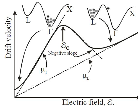
FIGURE 5.11 Illustration of the electron transfer from the  $\Gamma$ -valley to the L-valley in the conduction band of GaAs as the applied electric field is increased. The associated drift velocity behavior as a function of the electric field is shown with a negative slope on the right-hand side of the peak.
