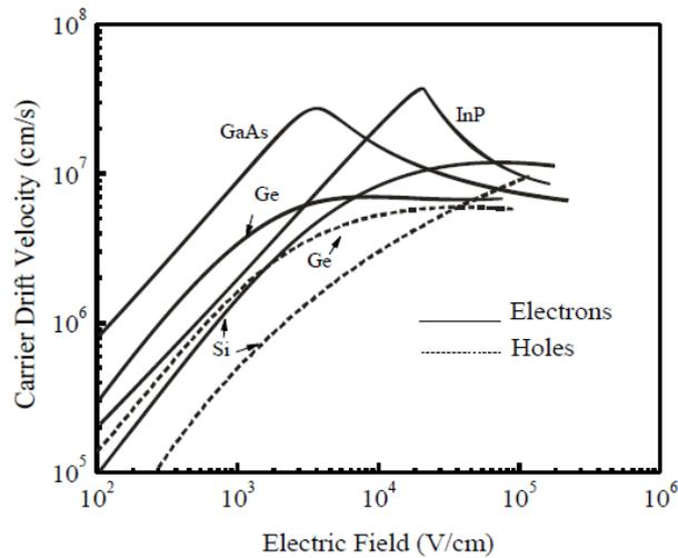
FIGURE 5.10 Carrier drift velocities as a function of the electric field for Si, Ge, GaAs, and InP.
