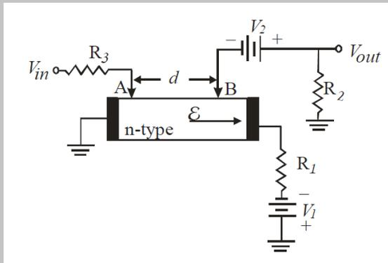
FIGURE 5.17 An illustration of the Haynes-Shockley experiment.
