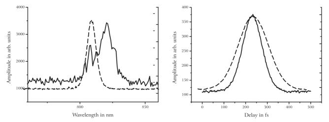
FIGURE 2 Left: input and output spectra at an output power of 1.16 mW corresponding to a pulse energy of 14.1 pJ. Right: corresponding autocorrelation traces. The dashed curves show the input pulse, the solid curves the output pulse after the fibre
