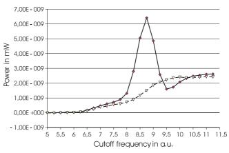
FIGURE 3 Typical measurement curve at a pulse energy of 15.8 pJ. The AC noise powers of sum (*solid line*) and difference (*dashed line*) photocurrents over the filter high-pass cut-off are given in arbitrary units
