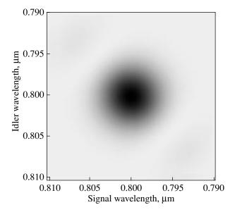
**Fig. 6.** Joint spectral intensity of the two-photon state produced by a sequence of ten BBO crystals and nine calcite spacers, as was discussed in the text. The plot shows the region of the main degenerate peak near  $\lambda_s = \lambda_i = 800$  nm.
