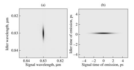
**Fig. 2.** High-aspect-ratio two-photon state obtained by degenerate collinear PDC of a pump pulse of approximately 100-fs duration at 415 nm in a 2-cm-long KDP crystal. The state exhibits space–time decorrelation. (a) Factorable joint *spectral* intensity; (b) factorable joint *temporal* intensity.
