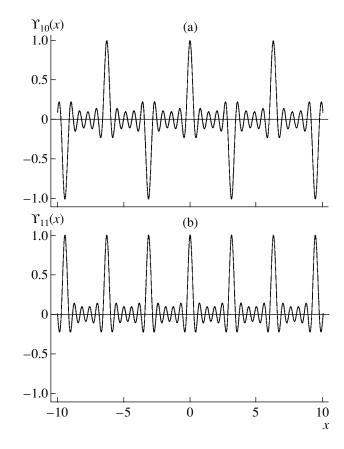
Fig. 4. Plots of the  $\Upsilon_N(x)$  function showing different behavior for even and odd N; while for even N peaks alternate with valleys (separated by  $\pi$ ), for odd N there are no valleys. The peaks and valleys become narrower with increasing N. Such a function describes the phase-matching contribution from the crystal birefringent spacer sequence.
