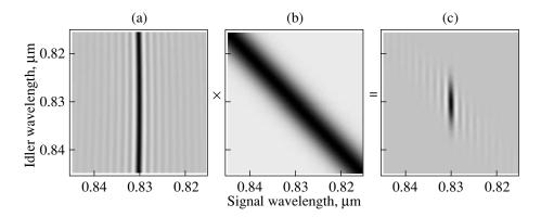
**Fig. 1.** High-aspect-ratio decorrelated two-photon state obtained by degenerate collinear PDC from a 2-cm-long KDP crystal exhibiting a cut angle of 68°. (a) "Vertical" phase-matching function  $\phi(\omega_s, \omega_i)$  exhibiting asymmetric group velocity matching. (b) Pumpenvelope function describing a Fourier-transform-limited pump pulse centered at 415 nm with a spectral bandwidth of 5 nm. (c) Resulting nearly factorizable two-photon state.
