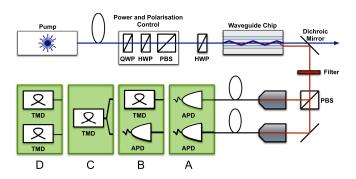
FIG. 1 (color online). Scheme of experimental setup (see text); measurement configurations A, B, C, and D provide information about detector efficiency, marginal and collective statistics, and joint correlations, respectively.
