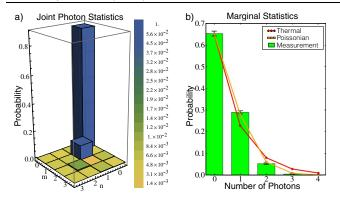
FIG. 3 (color online). (a) Joint photon statistics  $p_{n,m}$  measured with two TMDs and pump power of 220 nW. (b) Marginal statistics of idler with pump power of 375 nW. The measurement is fitted against thermal and Poissonian distributions.
