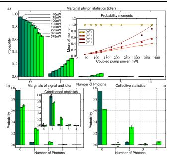
FIG. 2 (color online). (a) Marginal photon number statistics in idler mode for various pump powers; Inset: first probability moments  $\langle n^m \rangle$  with a fit to a Poissonian distribution. (b) Comparison of signal and idler marginals for lowest and highest pump power; Inset: conditioned statistics demonstrate vacuum suppression. (c) Collective photon pair statistics (see text) for lowest and highest pump powers.
