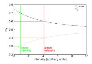
FIG. 3. (Color online) The mode occupation probabilities  $m_1$  and  $m_2$  for a single-photon event in dependence of the pump intensity.
