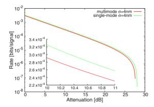
FIG. 4. (Color online) Solid (red) line: lower bound on the secure key rate for the KTP crystal with a pump width of 4 nm. Dashed (green) line: lower bound on secure key rate for the same photon number distribution, but with all photons in the same spectral mode. The inset shows a zoom of the 10–11 dB region. The weak decoy mean photon number is 0.1 in both cases, and the signal mean photon number is optimized to result in the largest possible rate.
