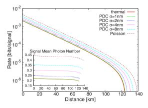
FIG. 5. (Color online) Lower bound on the secure key rate for different pump widths and therefore different mode contributions. The asymptotic cases are the rates for thermal and Poissonian distribution. The inset shows the optimized mean photon number of the signal state. The weak decoy mean photon number is fixed to 0.1 for all scenarios.
