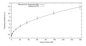
FIG. 4. Relation between pump power and coupling parameter. The expected square-root dependency [11] is correctly obtained for a wider range of pump intensities than can be resolved with current TMDs, which ensures the validity of our approach also for high powers. Notice that this knowledge would also allow for computing the expected mean photon number for a given pump power or a determination of  $\chi^{(2)}$ , as described in [23].
