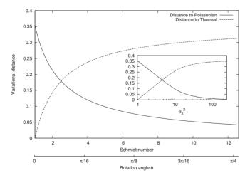
FIG. 2. Solid line and dashed line show the distance between the convoluted photon number distribution and Poissonian or thermal statistics, respectively, plotted against the Schmidt number. For a single effective mode, the distribution is exactly thermal, but the more modes contribute, the closer it gets to a Poissonian distribution. The inset fixes  $\theta = \pi/4$  and varies  $\sigma_x^2$ , which is drawn on a logarithmic scale.
