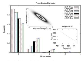
FIG. 3. (Color online) Comparison between experimentally measured and theoretically obtained photon number distributions for a multimode PDC process at various pump strengths. The bottom inset shows the real part of the joint spectral intensity, while the top inset demonstrates the parametrization of the analytical Gaussian approximation of the SDF. Loss inversion and error estimation was performed using non-negative least-squares optimization.
