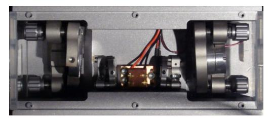
Figure 10 (online color at: www.lpr-journal.org) Picture of a bow-tie cavity with a PPKTP crystal used for squeezing the light field. The crystal is placed inside an oven (made of copper) which controls the crystal temperature to ensure optimal phase matching between the waves.
