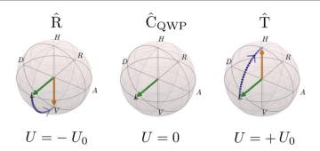
**Figure 5.** Bloch sphere representation of the EOM switching states corresponding to the three operations  $\hat{R}$ ,  $\hat{C}_{QWP}$  and  $\hat{T}$  exemplary for an horizontally polarised input state; a static QWP is placed in front of the EOM to realise  $\hat{C}_{QWP}$  in case no voltage is applied.
