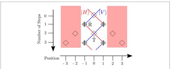
**Figure 3.** Illustration of how the spread of the walker's external state is limited via polarisation switching; a reflection  $\hat{R}$  is represented by a grey box and switches the horizontal (red lines) into vertical (blue lines) polarisation and vice versa. The transmission operation  $\hat{T}$  is represented by a white box leaving the polarisations unchanged. Note that in the setup the spatial position is in the experiment mapped into the time domain.
