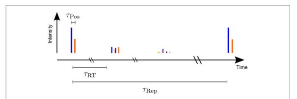
**Figure 2.** Schematic illustration of the three relevant timings (not to scale): the position spacing  $\tau_{Pos}$ , the roundtrip spacing  $\tau_{RT}$  and the time  $\tau_{Rep}$  between two consecutive experiments defining the repetition rate; counts for vertically polarised light are represented by blue bars and counts for horizontally polarised light by orange bars (schematically).
