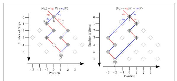
**Figure 17.** Illustration of the implementation of the 5 step state-transfer scheme (left) and the 6 step state-transfer scheme (right). For both schemes, the phase of *i* introduced by the reflection operation is compensated for by applying it four times.
