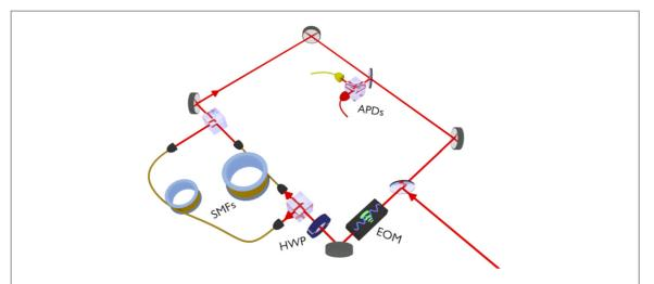
**Figure 1.** Schematic of our implementation of a time-multiplexed quantum walk with an electro-optic modulator (EOM) and a half-wave plate (HWP) (here exemplarily) carrying out the coin operation, two single mode fibres (SMFs) introducing the time delay and the avalanche photo-diodes (APDs) used for the read-out of the walker's state.
