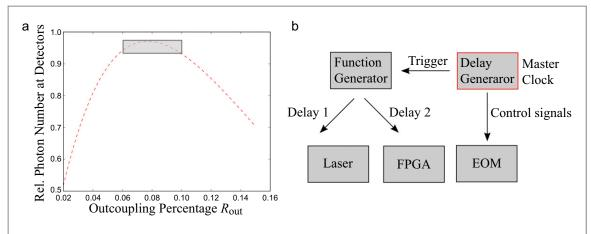
**Figure 7.** Left figure: the relative power at the detectors depending on the outcoupling percentage  $R_{\text{out}}$  for a step number of 13, the optimal values for reflectivities are marked by the grey box (between 0.06 and 0.10); Right figure: schematic of the components significant for the timings in the setup and the signals sent between them; FPGA: field-programmable gate array.
