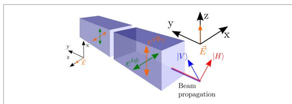
**Figure 4.** Schematic of the two EOM crystals; the reference frame is given by the orientation of the crystal axes and is rotated by 45° with respect to  $|H\rangle$  and  $|V\rangle$ : the phase  $\phi$  originating from the natural birefringence is accumulated along the x-axes, while the phase  $\Phi_U$  originating from the application of  $\vec{E}$  is accumulated along the z-axes of the crystals.
