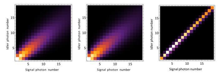
FIG. 2. An experimentally obtained JPD (left), a reconstructed JPD (center), and an initial JPD of a generated light state in the absence of losses. Fit parameters are {thermal<sub>1</sub>,  $\mu_1 = 18.98$ ; thermal<sub>2</sub>,  $\mu_2 = 0.93$ ;  $\eta_s = 0.44$ ;  $\eta_i = 0.53$ ; Poisson<sub>s</sub>,  $\mu_s = 0.07$ ; Poisson<sub>i</sub>,  $\mu_i = 0.21$ }, quality of the fit is characterized by *P* value obtained for Pearson's  $\chi$ -squared test and equals 0.999 999.
