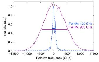
**Figure 3 | Marginal spectra before and after conversion.** Marginal spectra of the PDC idler photon before (magenta) and after (blue) frequency conversion in the quantum pulse gate centred around their respective centre frequencies. Dashed lines correspond to Gaussian fits from which the bandwidths were obtained. The spectrum of the idler photons were measured using a dispersive-fibre time-of-flight spectrometer. A Czerny-Turner spectrograph was used for the spectrum of the converted light.
