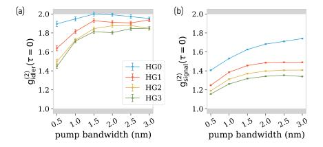
Fig. 8. The second-order correlation measurements of the idler and signal photons with the pump set to different bandwidths and different orders of Hermite-Gaussian modes. The error bars for the  $g_{\text{signal}}^{(2)}(\tau = 0)$  are smaller than the markers.
