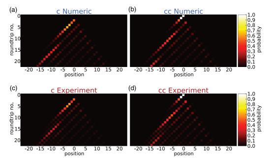
FIG. 10. Numeric and experimental evolution of intensities of each traveling direction in a Hadamard walk with partial reversal of the c and cc traveling directions, initialized in  $|ccA\rangle$ . The sum of the two intensity distributions yields the distribution of a standard Hadamard walk. The averaged similarity between numeric and experimental results over 22 steps is 93.1%.
