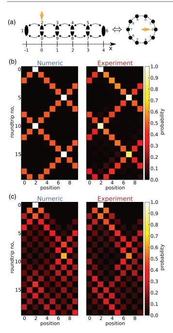
FIG. 7. (a) Configuration of an asymmetric circle walk on 10 sites. The walk is started at x = 0 (orange arrow), which corresponds to position m = 2 on the circle and in the chessboard plot axes. The input state is  $|ccV\rangle$  and (b) shows the step evolution of a nonmixing walk (similarity averaged over 19 steps:  $\bar{S} = 88.9\%$ ), while (c) displays the evolution of an effective Hadamard walk in such a configuration (similarity:  $\bar{S} = 79.9\%$ ).
