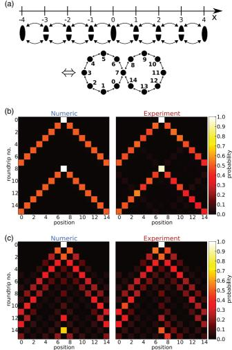
FIG. 9. (a) Modified ladder graph, equivalent to a walk on a figure-eight, shown here for a graph with 15 nodes. Note the coupling at x = 0, which involves all four possible links. (b) Numerics and experimental data of the intensity evolution of a figure-eight quantum walk with a nonmixing coin and  $|ccV\rangle$  input. The polarization resolved similarity averaged over 15 steps is  $\bar{S} = 90.3\%$ . (c) Same as (b) but with effective Hadamard splitting. (Similarity  $\bar{S} = 90.5\%$ )
