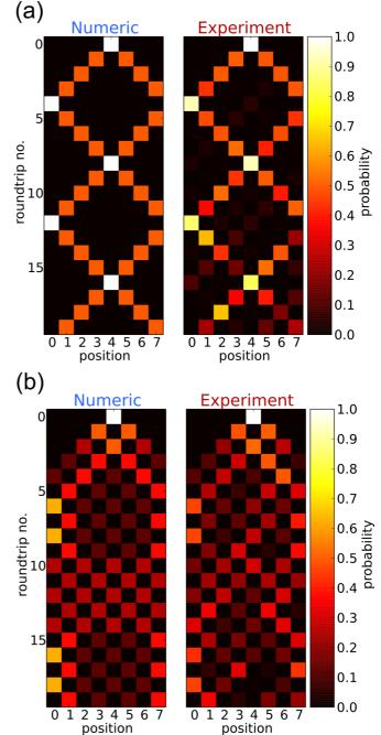
FIG. 14. 8-site circle (see Fig. 11): (a) free passage walk with a similarity  $\overline{S} = 85.5\%$  and (b) Hadamard-like H' walk with  $\overline{S} = 78.8\%$  (both averaged over 19 steps) with  $|ccV\rangle$  input.
