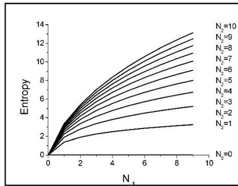
**Fig. 25.7** The entropy production function  $F(N_1, N_2)$  in eq.(9) is plotted versus  $N_1$  in the range from 0 to 10. The parameter  $N_2$  is in the range from 0 to 10.
